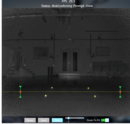
Figure 2.6: Scene calibration: Calibration markers in green are labeled (sagittal view). Walking line is defined between the start and end points, shown in red.
