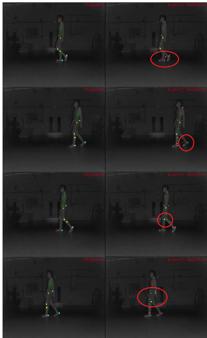
Figure 2.1: Sagittal View Motion Capture using ‘OPTIKA’ and MS Kinect v2. The captured joints in infrared images are shown in unique colors. Comparing the results of the tracking results from ‘OPTIKA’ and Kinect v2 shown in the first and second columns, this figure demonstrates the tracking failures of front panel foot , back panel foot , knee joint , waist from the first to last row, respectively.
