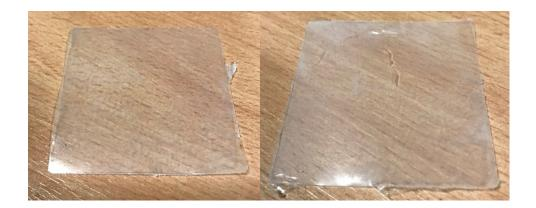
Figure 3.6 Thin film samples produced by using a press machine.
