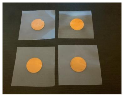
Figure 5.2 Thin film samples for dielectric spectroscopy.
