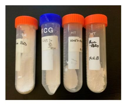
Figure 3.3 Nanoparticle powders with and without surface modification.
