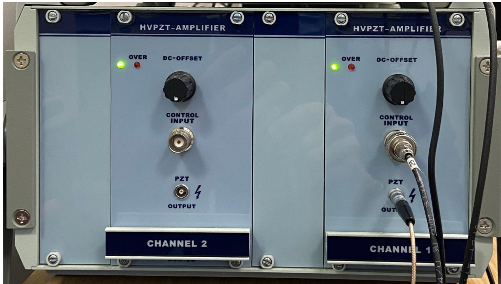
Figure B-1. Schematic of CoreMorrow E01.A2 power amplifier.
