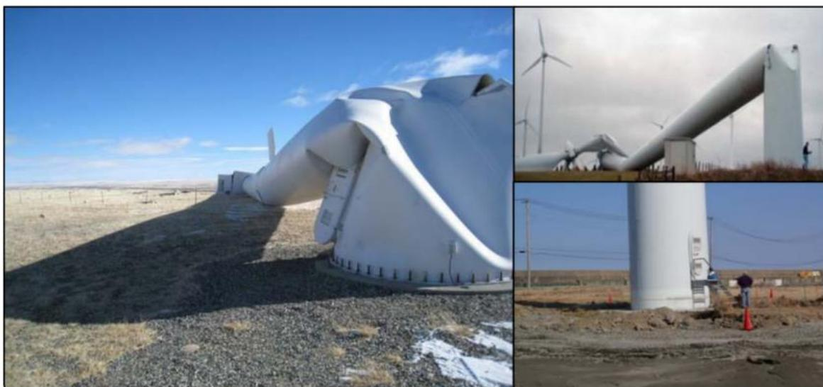
**Figure 1.2** Wind turbine collapse due to ground-shaking in Japan (left) and New Zealand (right). Taken from Asareh (2015).
