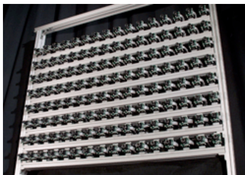
(a) The 128 video cameras are arranged 2 inches apart to simulate a single camera with an aperture 3 feet wide.
