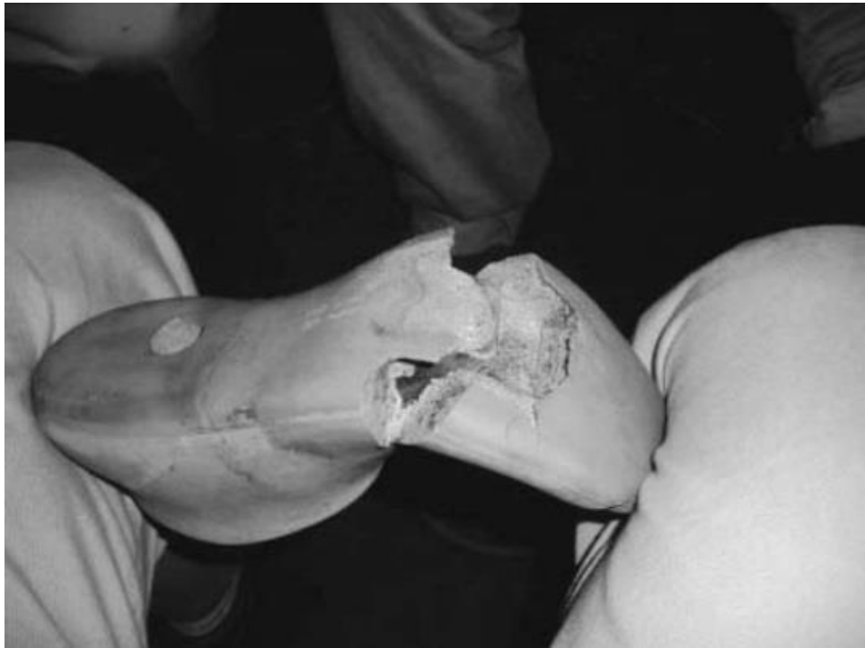
Figure 25 – Fracture of the forefoot of the Strider (Jensen, Nilsen, Thanh, et al., 2006)
