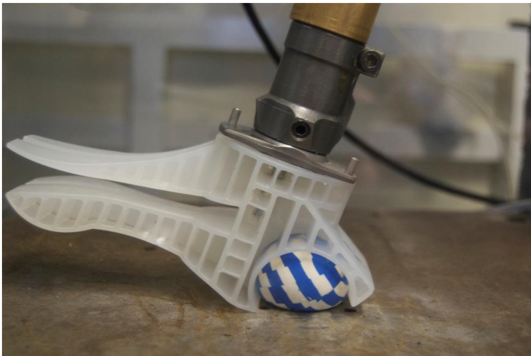
Figure 39 – An image showing sample 2 under maximum P3 heel loading showing contact of keel and baseplate
