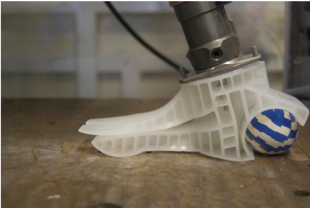
Figure 43 – An image showing sample 1 of the Strathclyde foot under maximum P4 toe loading
