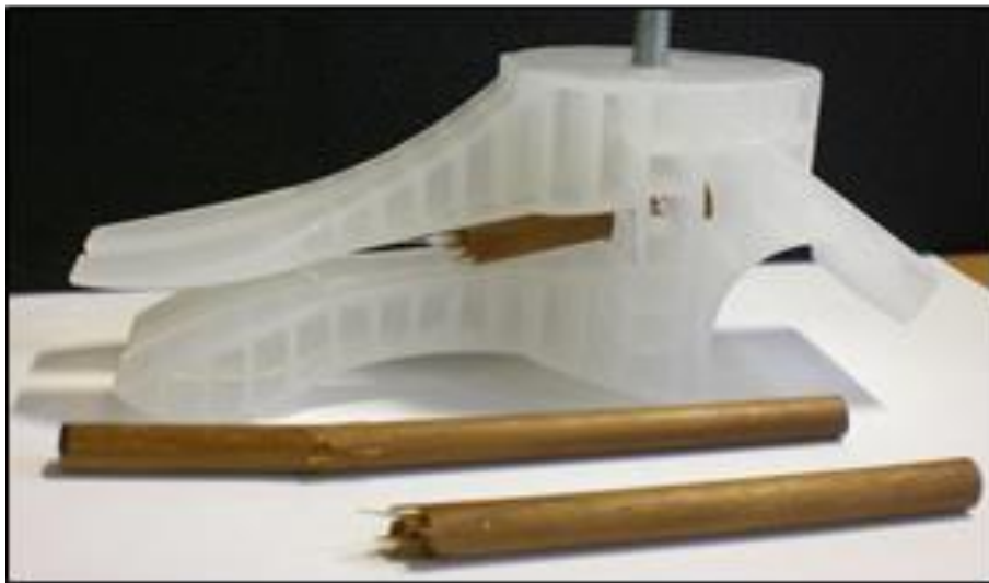
Figure 60 – Strathclyde foot showing the inserted threaded fastener used in previous testing (L. E. Morton et al., 2009)
