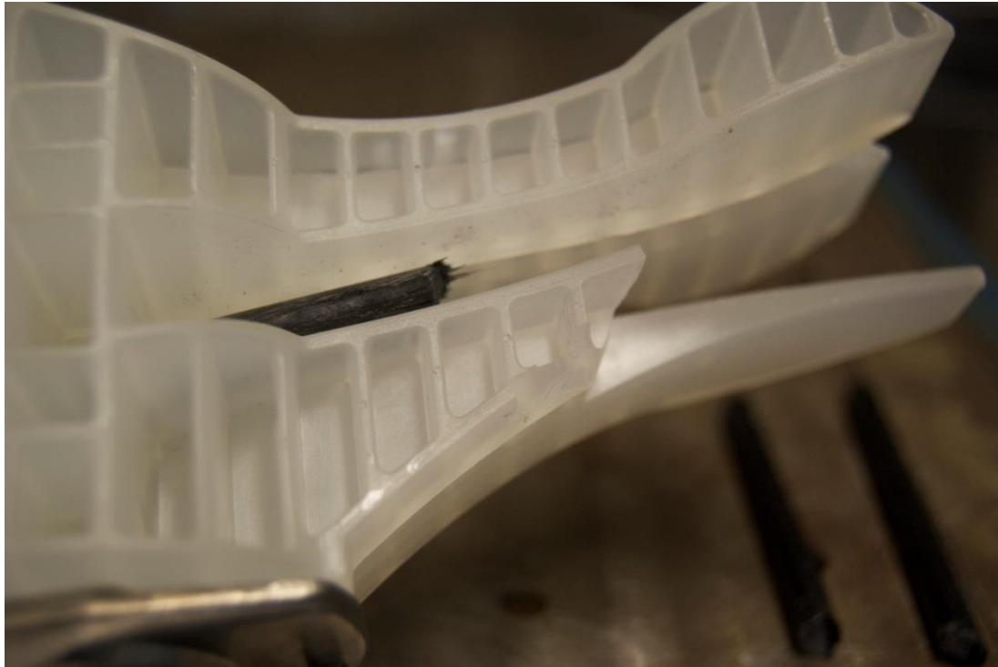
Figure 37 – An image of sample 3 showing the broken toe section and rods following P3 testing
