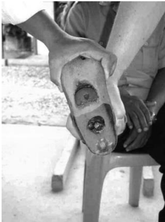
Figure 14 – Penetration of the keel of the VI-Cavity foot (Jensen, Nilsen, Zeffer, et al., 2006)
