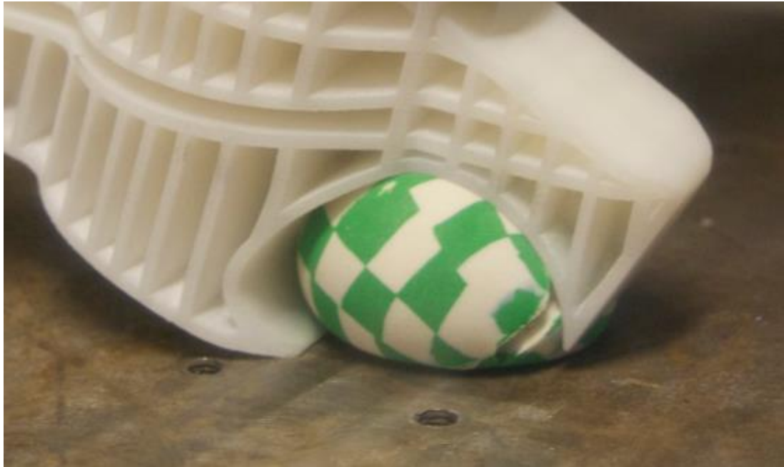
Figure 113 – Sample 1 under maximum P3 heel loading condition displaying the split in the ball
