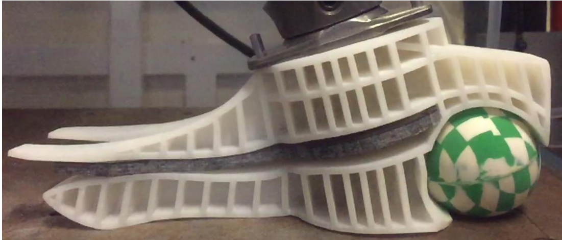
Figure 98 – Sample 4 at maximum load during P5 toe testing
