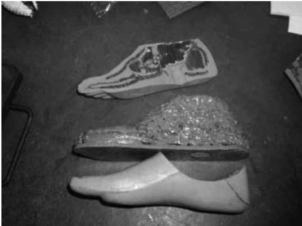
Figure 11 – A cross section of the VI-Solid foot showing the internal makeup (Jensen, Nilsen, Zeffer, et al., 2006)
