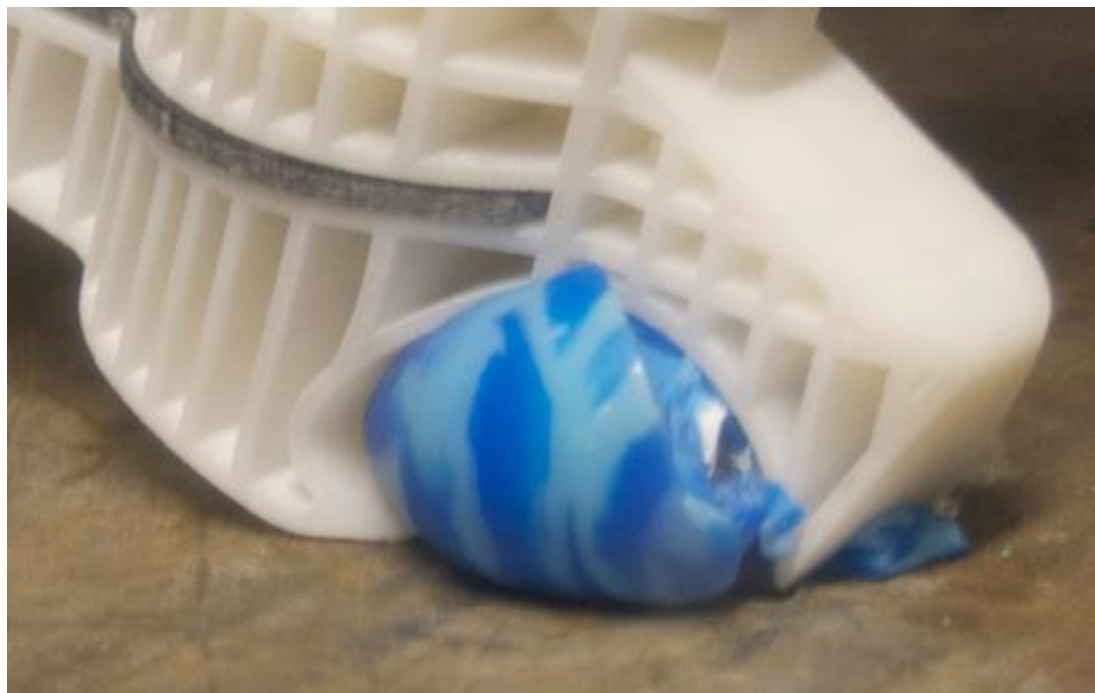
Figure 114 – Sample 2 under maximum P3 heel loading condition displaying the ruptured ball
