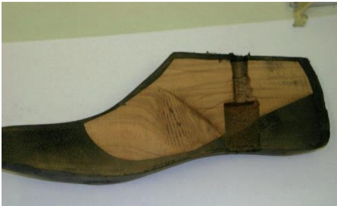
Figure 126 – Cross section of a Tatcot foot (from Jensen & Treichl, 2007(Jensen & Treichl, 2007))
