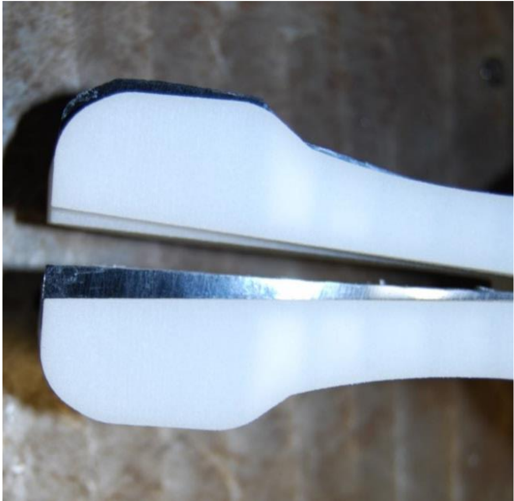
Figure 111 – The blade slipped to the right side during the P3 toe loading test
