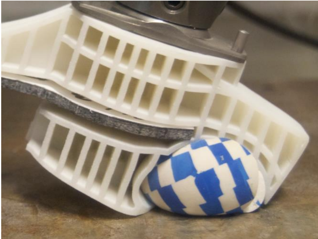
Figure 93 – Sample 3 showing the split ball under maximum P4 ultimate static load
