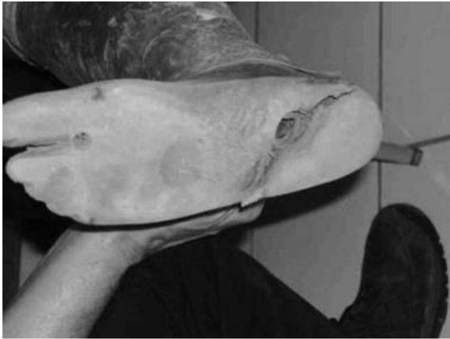
Figure 13 – Fracture of the sole of a VI-Cavity foot (Jensen, Nilsen, Zeffer, et al., 2006)
