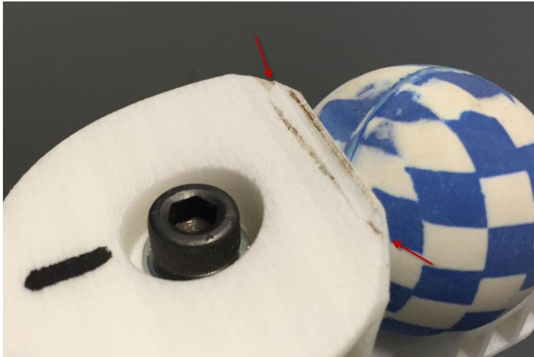
Figure 86 – An image showing the fracture in sample 1 from P3 heel testing. Arrows indicate the edges of the dark line highlighting the break
