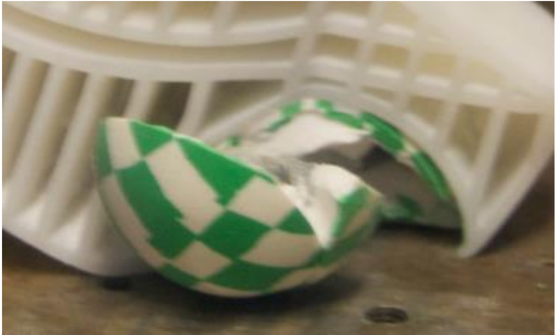
Figure 117 – Image showing the ruptured heel ball during P4 ultimate static loading heel testing
