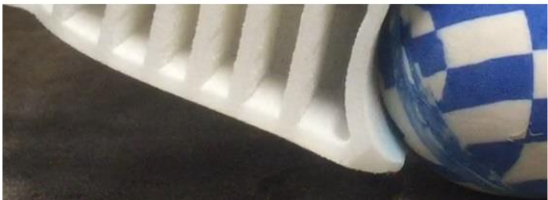
Figure 97 – Comparison of sample 2 pre- and post- P3 heel testing showing the deformation of the keel section
