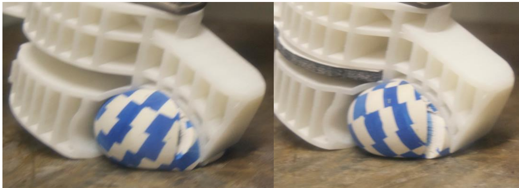
Figure 101 – Sample 2 (left) and sample 3 (right) showing the split balls at maximum load
