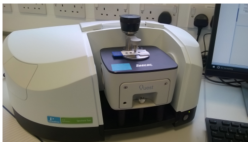
Figure 3.2: The Spectrum 2 FTIR spectrometer with Quest accessory and SIREs
