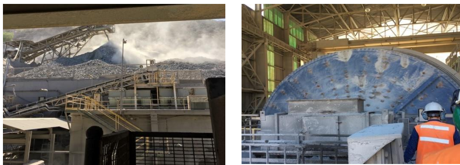
Figure 1. Minerals leaving a conveyor after a series of crushing (left) and the SAG mill (right).
