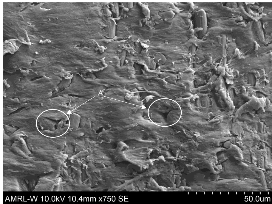
Figure 154. Details of wear scar Nylon 12CF 45,0 impingement angle with epoxy sealed surface, x750 magnification.
