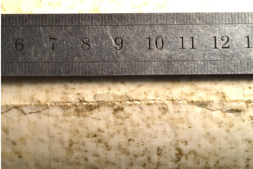
Figure 75. Image of brittle failure on the outside of the ABS cylinder.
