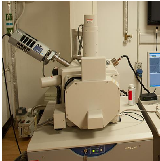
Figure 103. HITACHI S-3700, a variable pressure, tungsten filament, large chamber 300mm x 110mm, scanning electron microscope.
