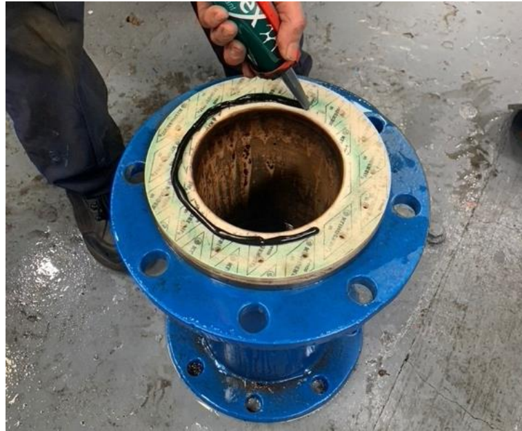
Figure 70. Application of liquid rubber to aid in sealing ABS cylinder for pressure testing.
