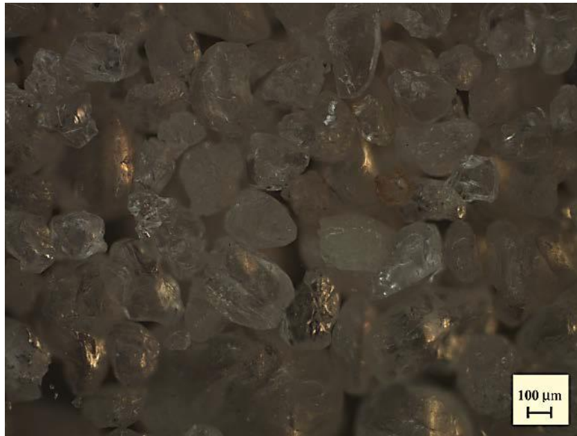
Figure 99. Angular silica sand used for testing with a size range of 355-500 \mu\text{m} [3].
