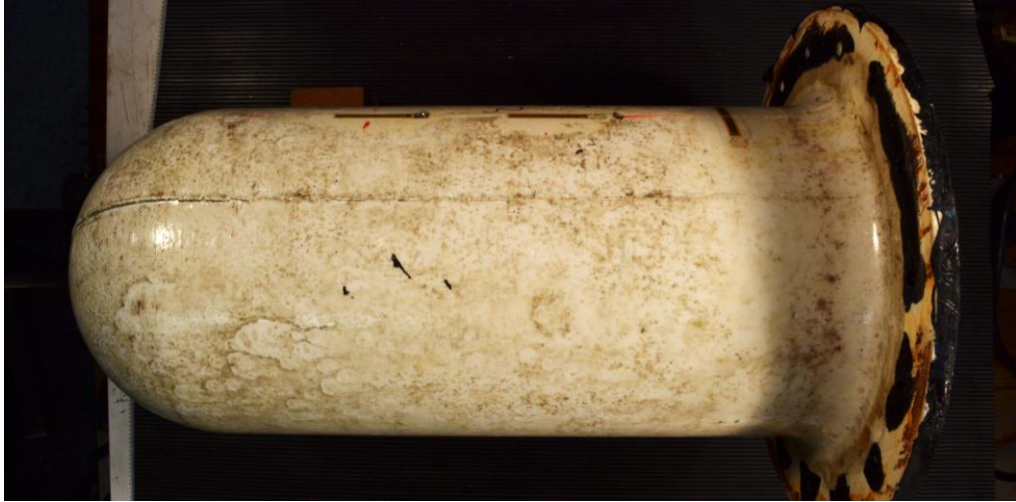
Figure 72. ABS cylinder crack along axis.
