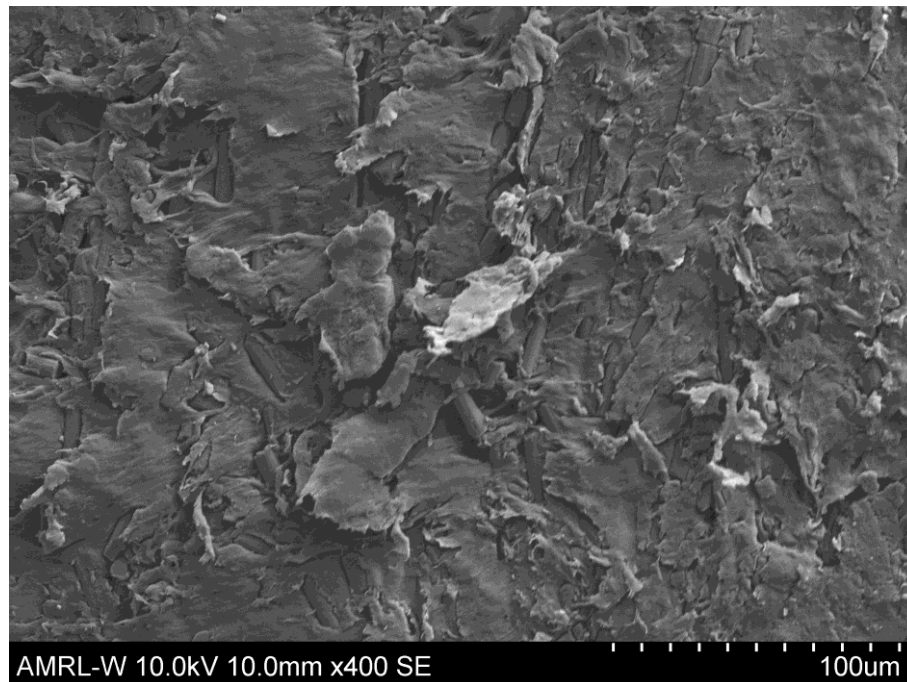
Figure 151. Edge of wear scar for Nylon 12CF 45,90 impingement angle with epoxy sealed surface. x400 magnification.
