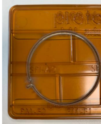
Figure 93. Ultem 1000 injection moulded placard showing water jet cut specimen for wear testing.
