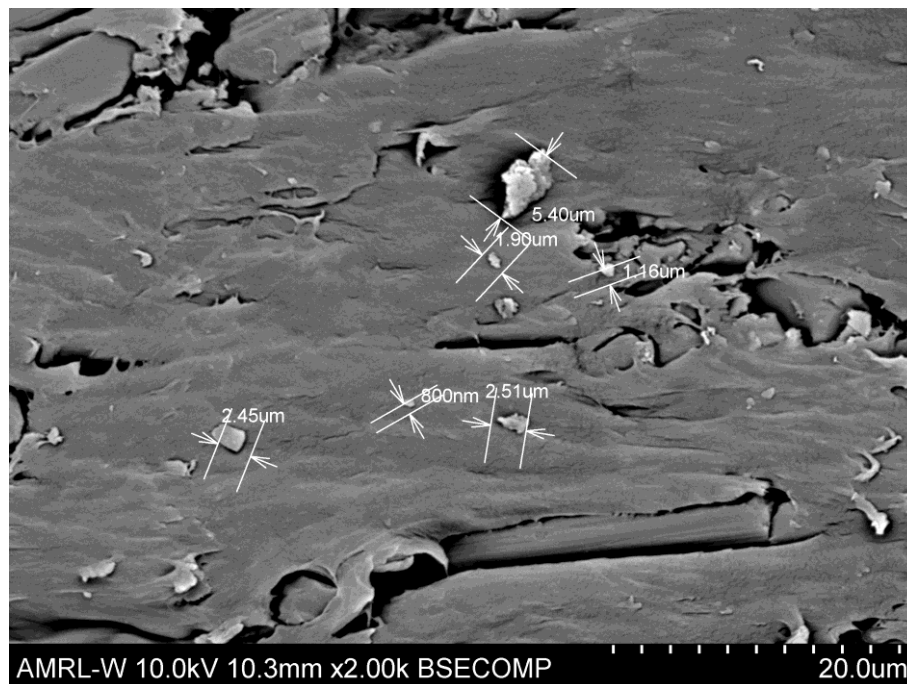
Figure 158. Sand found embedded in Nylon 12CF 45,0 impingement angle specimen with epoxy sealed surface, x2.00k magnification.
