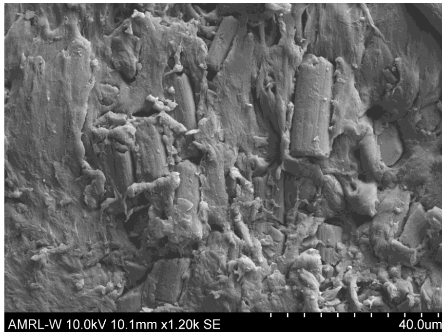
Figure 153. Exposed fibres at the edge of the wear scar Nylon 12CF 45,0 impingement angle. X1.20k magnification.
