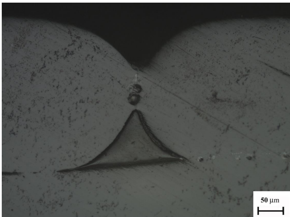
Figure 114. Sealed Ultem 1010 with epoxy visible between layers at x50 magnification.
