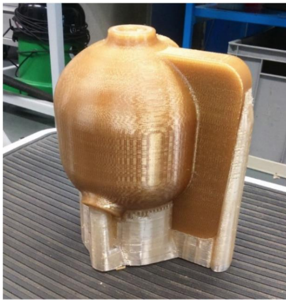
Figure 17. Printed model from ULTEM 1010 material on Stratasys Fortus 450mc [78].
