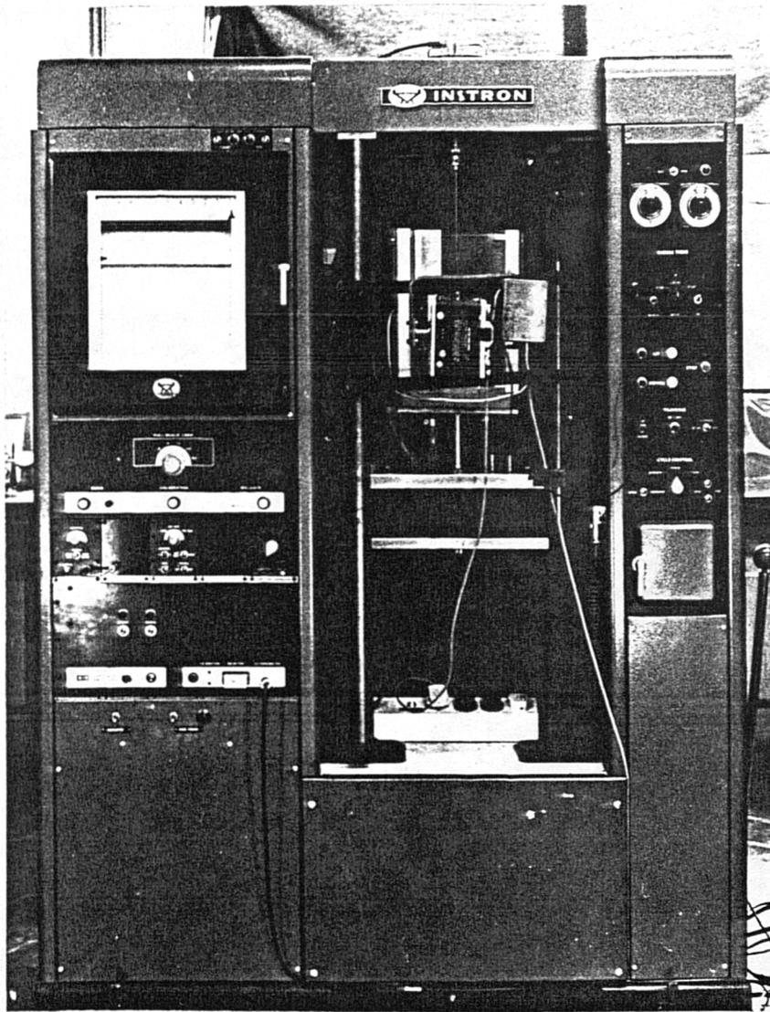
Fig IV.11 The Instron TT-CM Tensile Testing Machine
