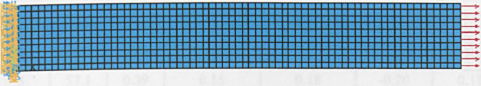
Fig 7.3: Plot of Boundary Conditions Used During Static Tensile Coupon FEA
