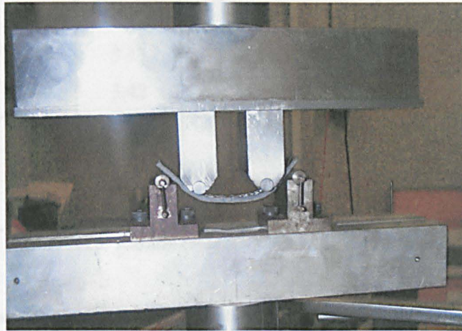
Fig 5.18: Photograph of Specimen During Flexure Testing
