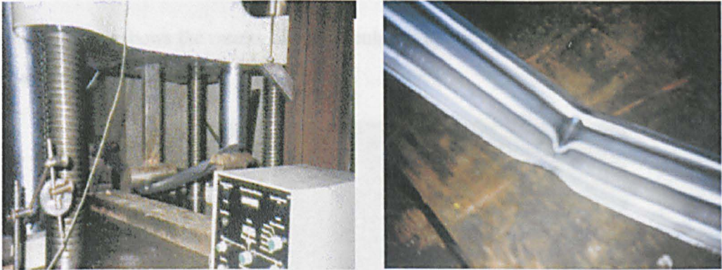
Fig 3.6: (a) Beam at Advanced Stage of Static Testing & (b) Local deformation
