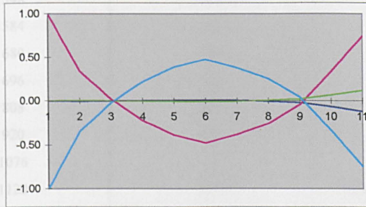
Fig A3.24 (a) Complex FRF Data at 232 Hz for the standard beam
