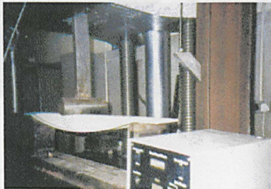
Fig 6.2: Composite Beam Prior to Static Testing
