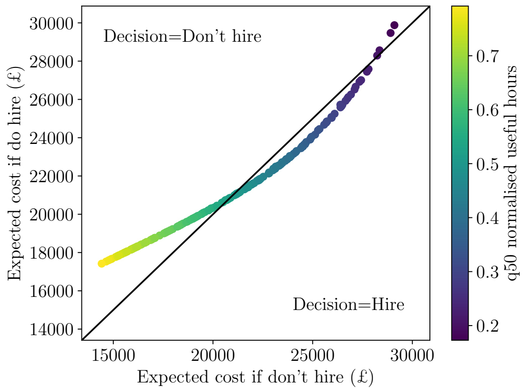
Figure 5.22: Expected cost of hiring crane, vs expected cost of not hiring crane, for 2-week ahead forecasts of number of available hours in the week. Colour shows the q50 forecast value of normalised number of hours within a weather window.
