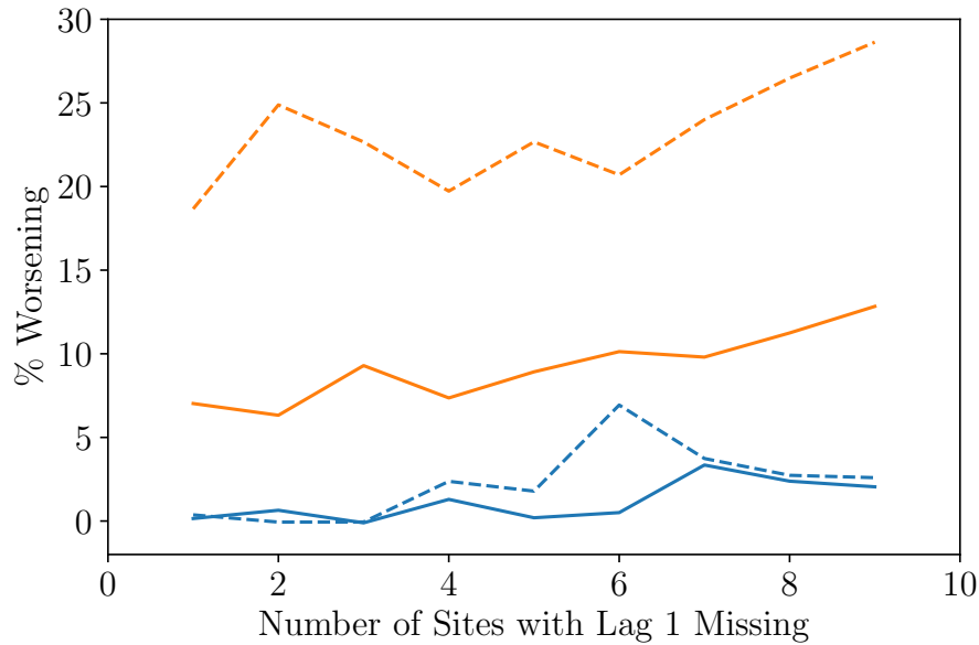
Figure 3.14: Case 4: Impact on forecast error of number of sites with lag 1 missing. The more sites missing data simultaneously, the worse the error, and the sites with data missing are most affected. Legend is the same as for Figures 1.11–1.13.
