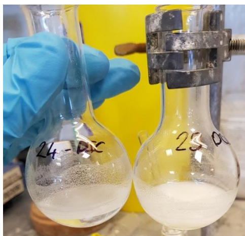
Figure 66. Photograph of the two larger-scale reactions between 5-phenyl-1 H -tetrazole 2-75 and 4-methoxybenzoic acid 2-78 . The flask on the left-hand side contains DIC as the coupling reagent and the flask on the right-hand side contains DCC. A difference in the amount of precipitate present can be seen with the diisopropylurea by-product being more soluble in organic solvent.
