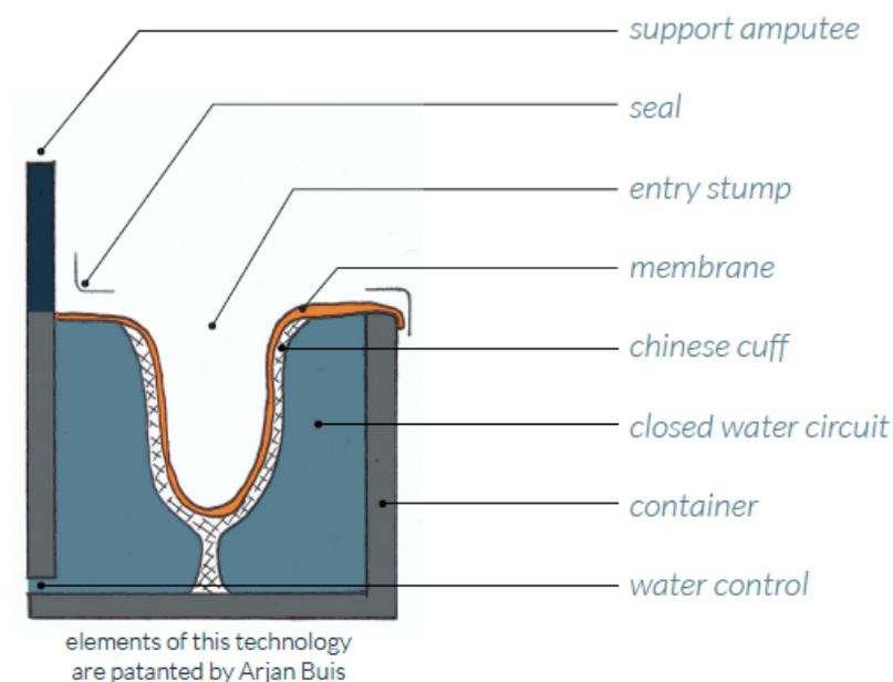
**Figure 3.** Schematic representation of the Majicast, which allows a cheaper method of production for lower limb prosthetic sockets. The use of water and the Chinese cuff device ensures a more uniform pressure distribution upon casting, creating a more suitable socket first time around and discarding the need for adjustments and a test socket (Joint Master Project, 2015).
