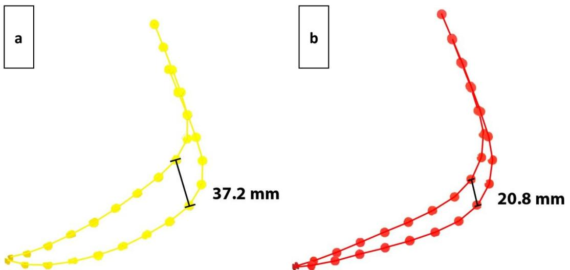
**Figure 23.** Quantification of the maximum deformation experienced by the carbon fibre (a) and natural fibre (b) forefoot during forefoot loading at test loading level P5. The carbon fibre forefoot shows a much more flexible characteristic than the natural fibre forefoot.
