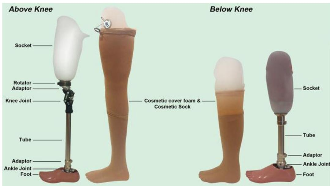
**Figure 1.** Image illustrating the components comprising an above-knee and below-knee prosthetic device. Both include the socket, the shin, the ankle joint with adapters and the foot with the addition of the knee joint and adapters for the above-knee prosthesis only. All these components can then be enclosed in a cosmetic cover (OrthocareIndonesia.com)
