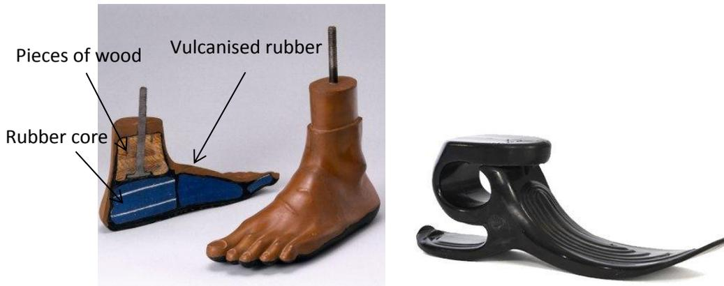
**Figure 4.** (Left) Image of the Jaipur foot illustrating the life-like look and a cross-section revealing the materials used for its manufacture (Cosgrove, 2013). (Right) Image of the Niagara foot manufactured entirely from Delrin and designed to provide a degree of energy return during gait (Suherman, 2012).
