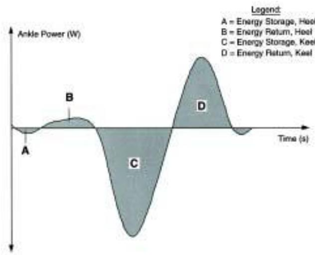
**Figure 7.** Power (W)–time (s) graph at the ankle that can be generated with the use of force plate and motion capture data. Area A and C represent the energy stored by the heel and keel respectively; area B and D represent the energy released by the heel and keel respectively (Hafner *et al.*, 2002).
