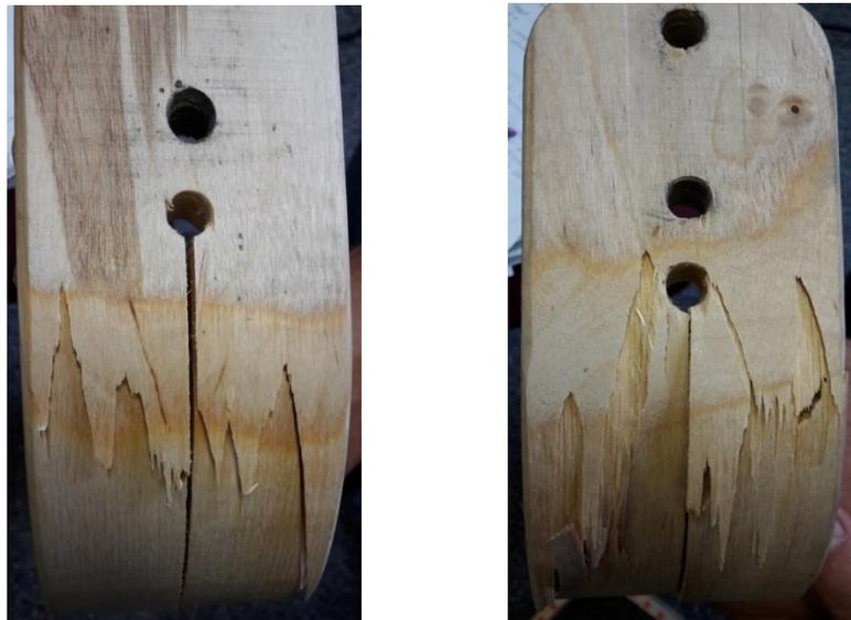
**Figure 26.** Image of the damage exhibited by the two 'optimised' natural fibre prosthetic feet with a thinner Baud curve (left) and a thinner toe section (right).
