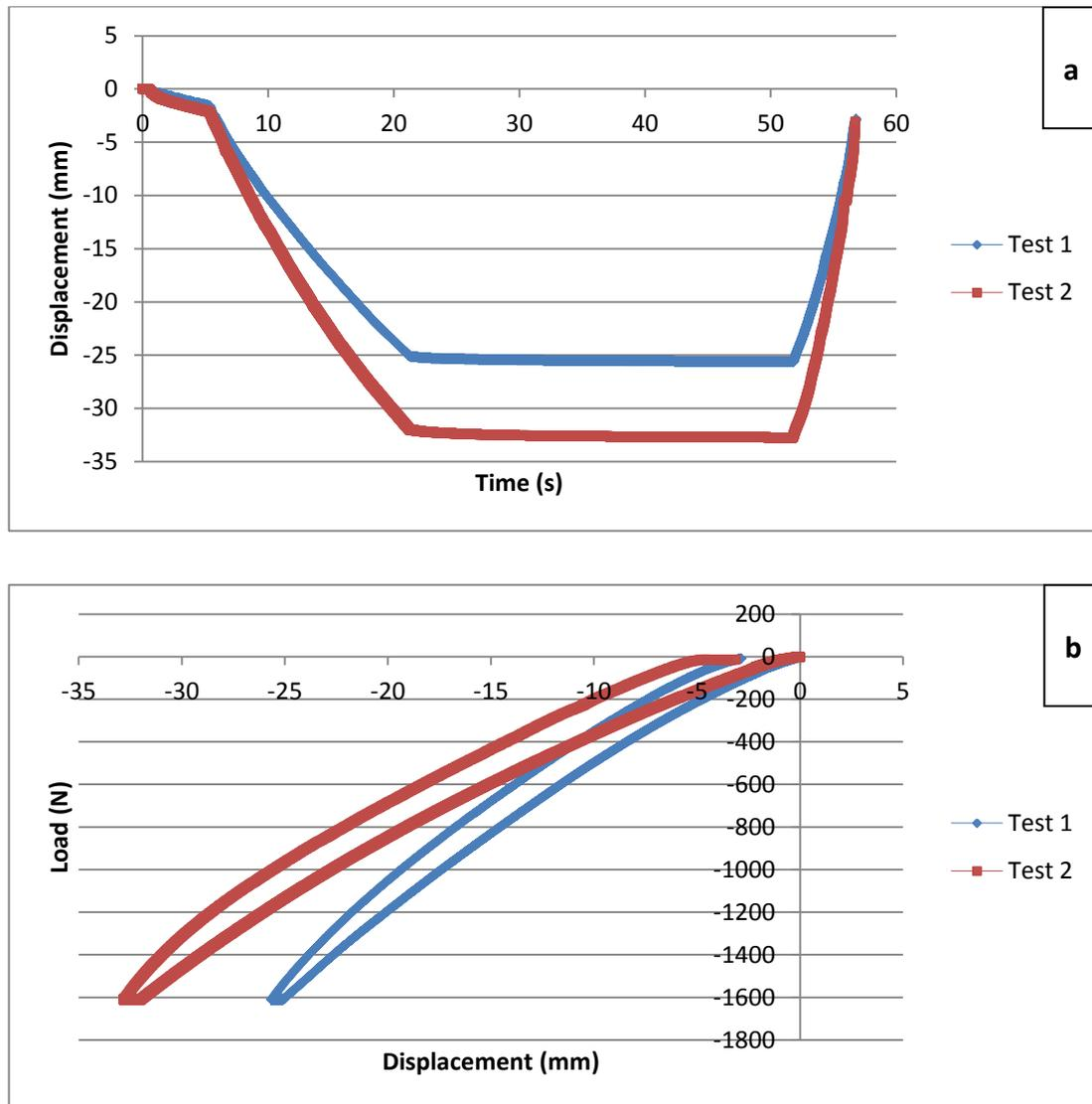
**Figure 19.** Comparison of the displacement (a) and energy efficiency (b) of the carbon fibre prosthetic forefoot at test loading level P3 for test 1 and test 2. Despite these two tests having been carried out on the same carbon fibre prosthetic foot, differences in displacement and thus stiffness were seen. The energy efficiency between the two tests did not show such difference.
