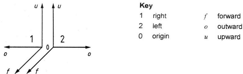
**Figure 10.** Coordinate system for right- (1) and left-sided (2) application and key as taken from BS EN ISO 10328:2006. *u*, *o* and *f* are the axes that run from the origin of the coordinate system in the proximal, lateral and anterior direction respectively.
