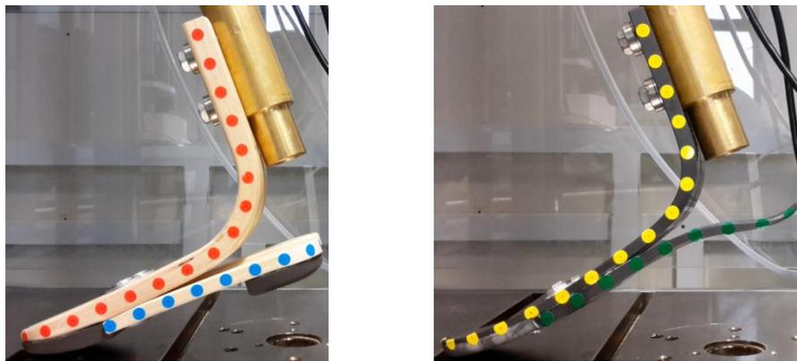
**Figure 14.** Picture illustrating the markers attached to the side of the natural fibre based composite prosthetic foot (left) and the carbon fibre prosthetic foot (right) at 20 mm intervals.
