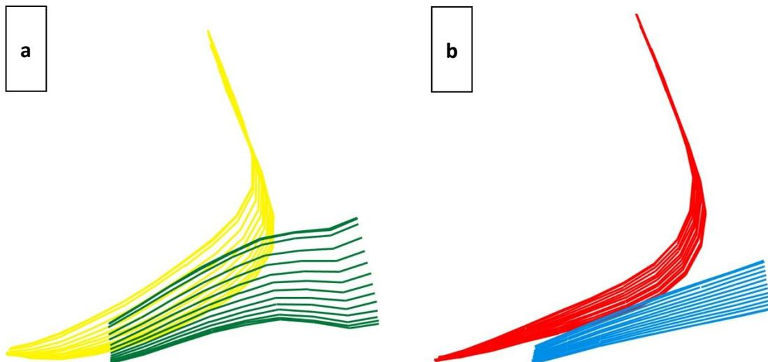
**Figure 22.** Deformation of the carbon fibre (a) and natural fibre (b) prosthetic foot during the loading period of the static proof test for forefoot loading at test loading level P5.
