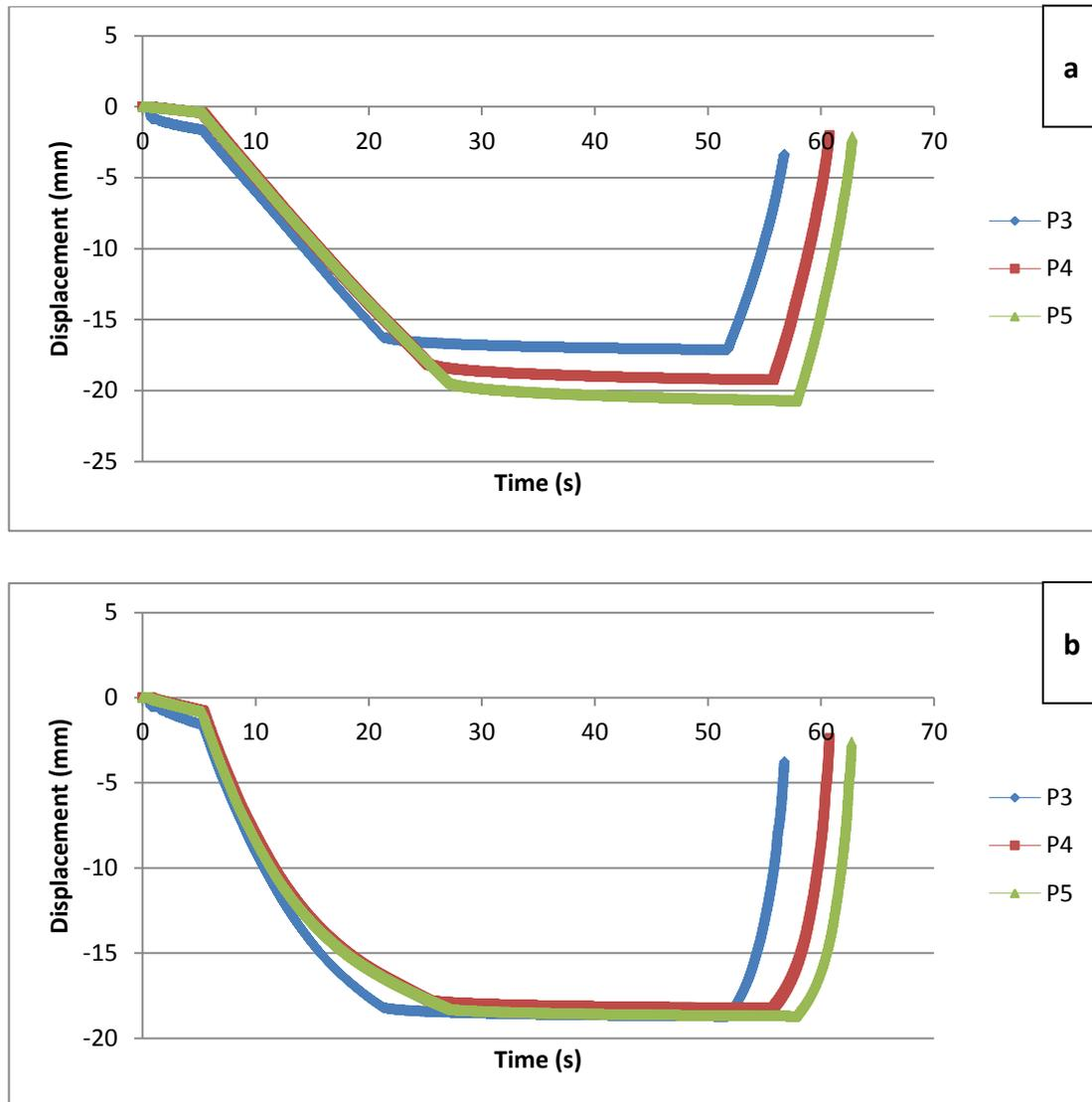
**Figure 20.** Comparison of the displacement of the natural fibre prosthetic forefoot (a) and heel (b) for test loading levels P3, P4 and P5, test 3. A gradual increase in displacement was seen from test loading level P3 to P5 with forefoot loading. However loading of the heel at increasing test loading levels did not result in any significant changes in displacement.
