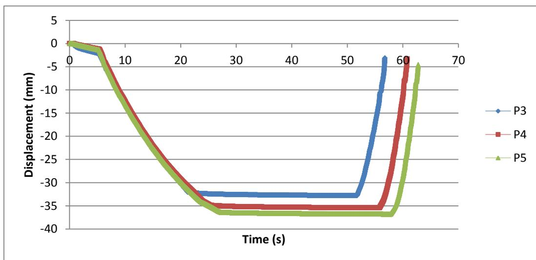
**Figure 18.** Comparison of the displacement of the carbon fibre prosthetic forefoot for test loading levels P3, P4 and P5, test 2. A gradual increase in displacement was seen from test loading level P3 to P5.
