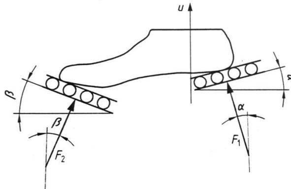
**Figure 11.** Schematic illustrating the angles of the forces to be applied to the prosthetic foot according to BS EN ISO 10328:2006, where  $\alpha = 15^\circ$ ,  $\beta = 20^\circ$ ,  $F_1$  = the force applied to the heel and  $F_2$  = the force applied to the forefoot (BS EN ISO 10328:2006).
