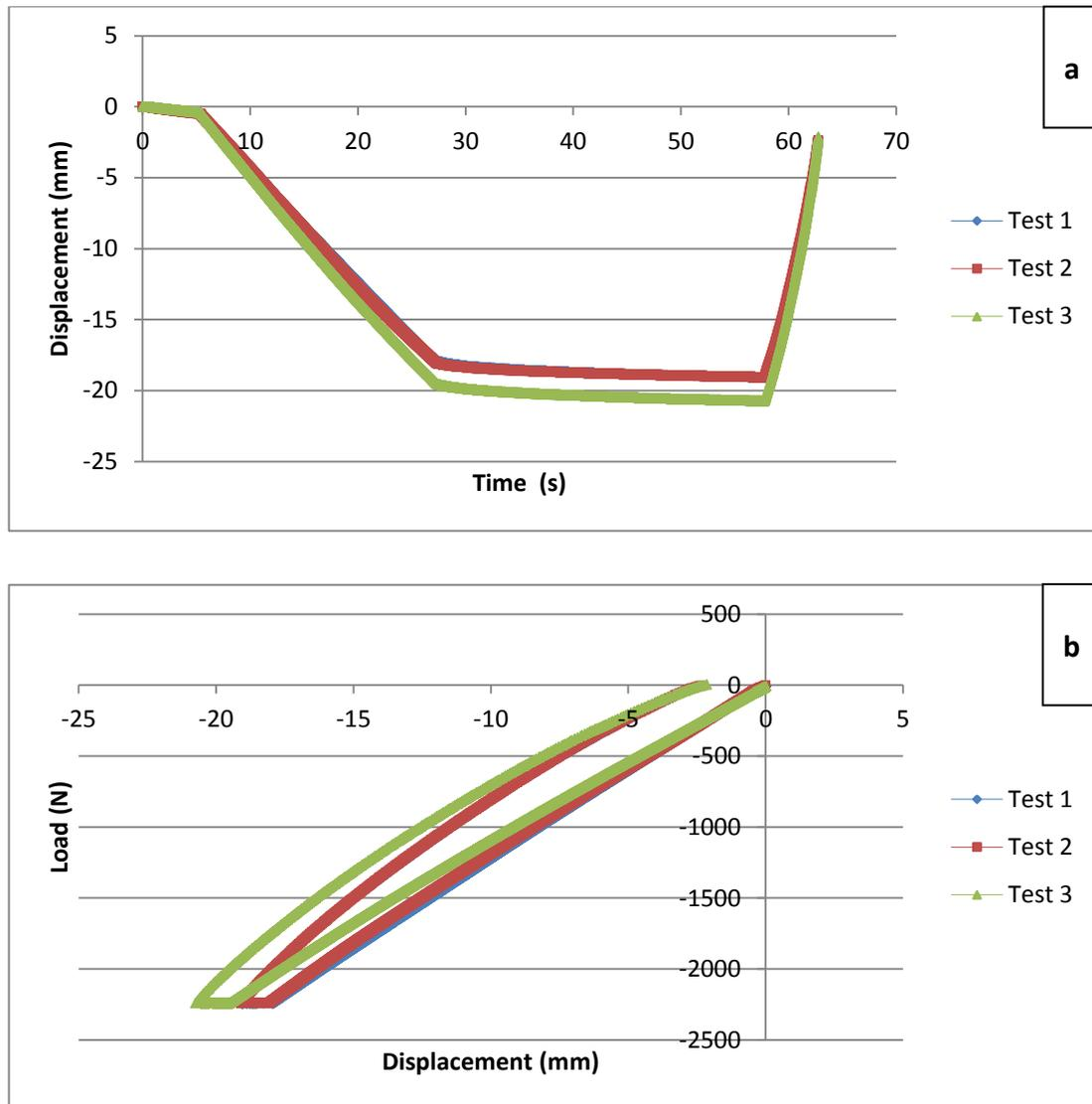
**Figure 21.** Comparison of the displacement (a) and energy efficiency (b) of the natural fibre prosthetic forefoot at test loading level P5 for test 1, 2 and 3. Only a slight variation was seen between the three different tests, with the energy efficiency remaining relatively constant.
