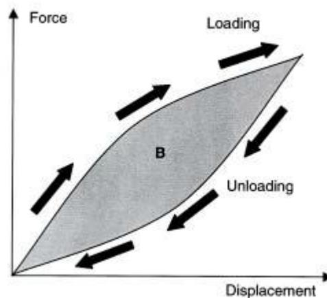
**Figure 8.** Graph of load against displacement that can be expected when loading and unloading a prosthetic device with an Instron machine. 'B' represents the energy dissipated by the prosthetic foot (Hafner et al., 2002).
