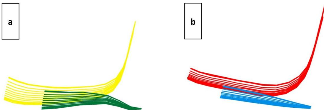
**Figure 24.** Deformation of the carbon fibre (a) and natural fibre (b) prosthetic foot during the loading period of the static proof test for heel loading at test loading level P5.
