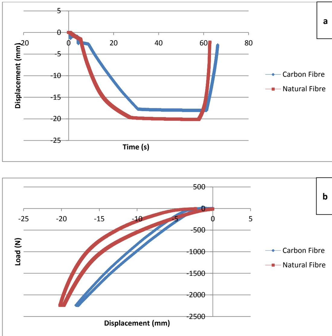
**Figure 17.** Comparison of the displacement (a) and energy efficiency (b) of the heel of the carbon fibre prosthetic foot and natural fibre prosthetic foot for test loading level P5, test 1. The natural fibre prosthetic foot showed a greater displacement with time. The carbon fibre heel displaced linearly with increasing load, whereas the natural fibre heel displaced less at higher loads.
