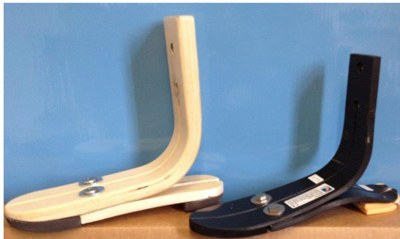
**Figure 9.** Image of the natural fibre based composite prosthetic foot prototype (left) and Össur's carbon fibre Vari-Flex prosthetic foot (right). The natural fibre prosthetic foot was constructed using a similar design to that of the carbon fibre type.
