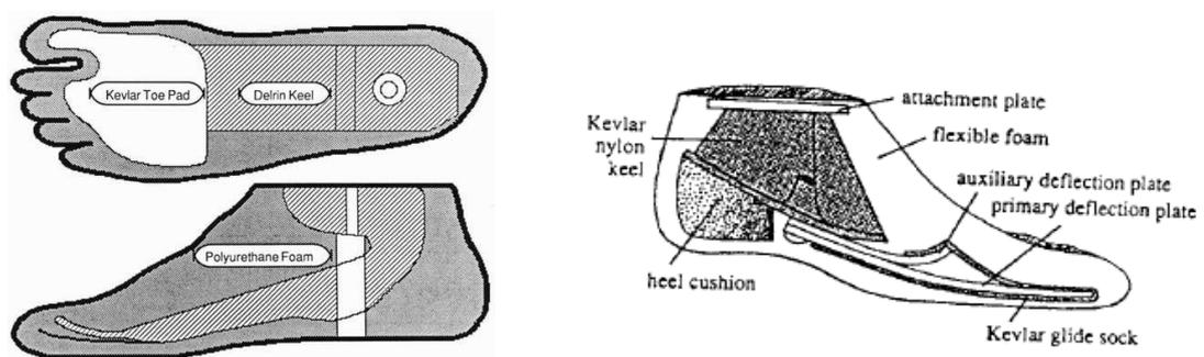
**Figure 5.** (Left) The Seattle foot consisting of a Delrin keel that acts as a cantilever spring for storing and releasing energy and a flexible Kevlar toe pad contained in polyurethane foam (Michael, 1987). (Right) The Carbon Copy II prosthetic foot with two deflection plates that allow for a two-staged resistance at heel-off (van Drongelen, 2000).
