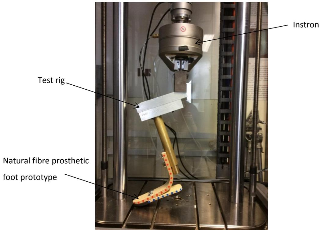
**Figure 13.** Image of the set-up for forefoot testing of the natural fibre prosthetic foot according to BS EN ISO 10328:2006. The prosthetic foot was attached to a metal test rig and clamped in the Instron with the desired angle of 20°.
