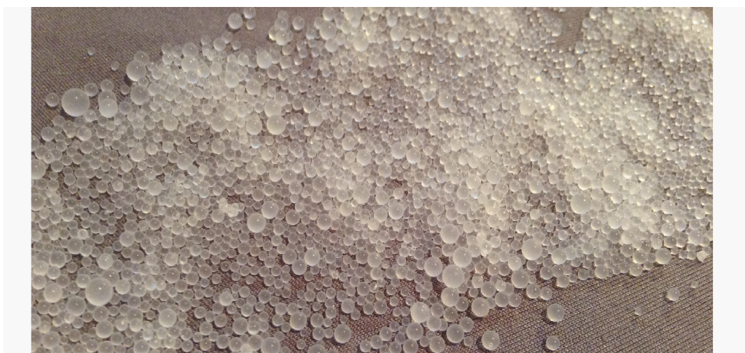
Figure 3.1 Polystyrene beads produced by suspension polymerisation reaction
