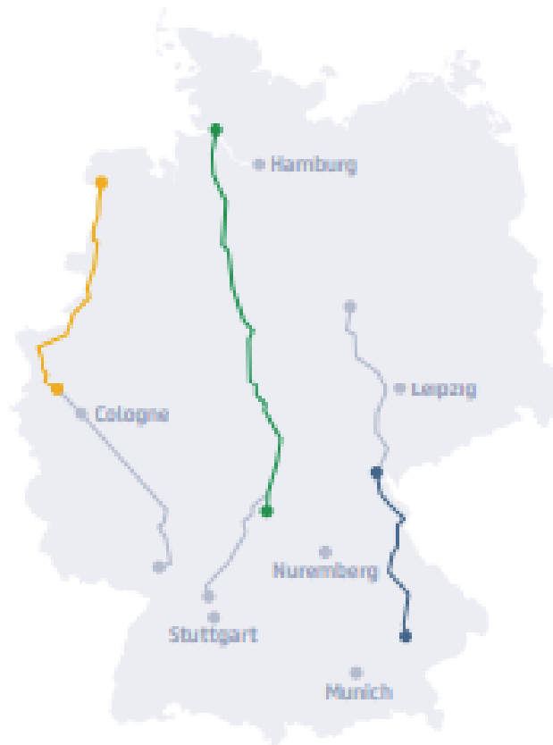
Figure 3.1: German HVDC transmission projects supporting large-scale renewable energy integration [1].
