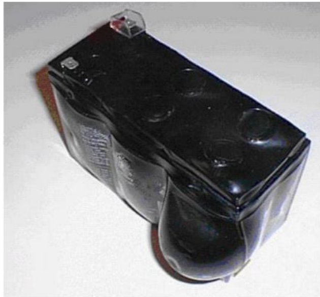
Figure 7 VRLA battery showing runaway conditions (Figure reprinted from Hoff et al. [60]).
