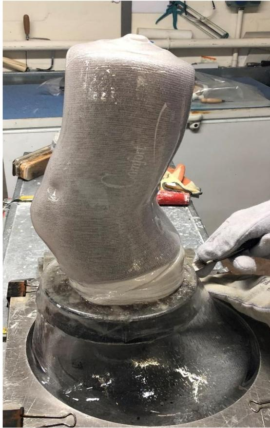
*Figure 26: Completed socket pre-machining*
