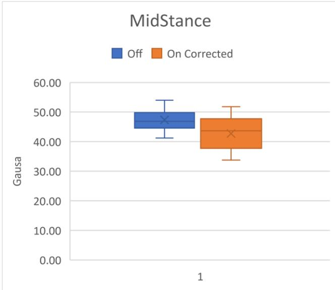
Figure 57: Box plot showing the Gauss measurement at Midstance with the device disengaged versus engaged.
