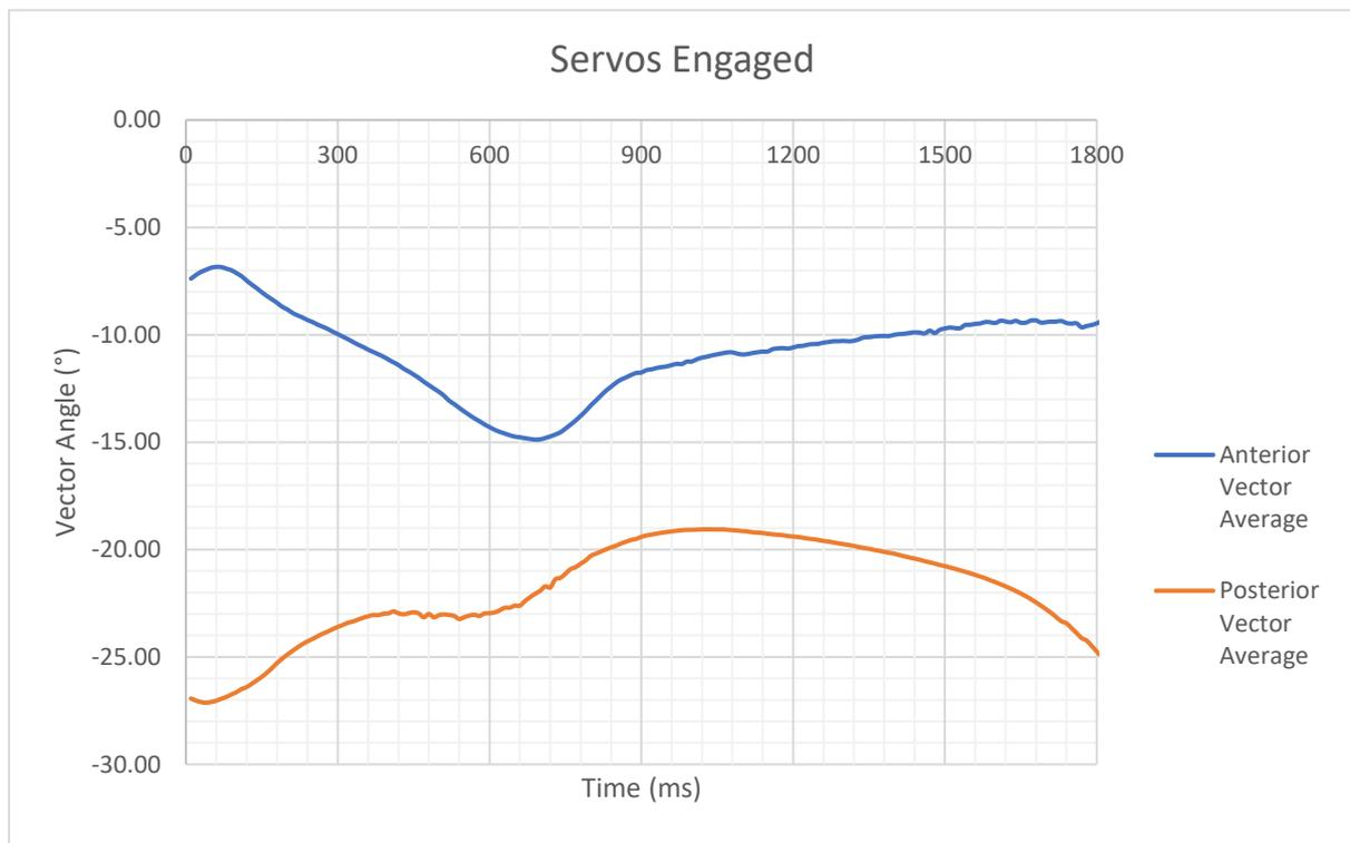
Figure 61: Anterior and Posterior vector angles calculated from data derived from the Motek CAREN system while the servos were engaged.
