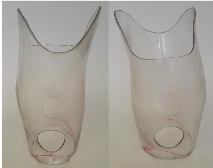
*Figure 27: Final, machined, open ended socket used to develop the initial prototype orthotic device for trials*
