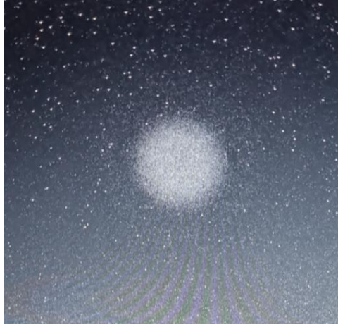
Figure 5.3: The screenshot of a collimated signal beam output of the Type-II collinear SPDC process seen on a CCD camera. The output is a Gaussian with waist of a 466 \mu\text{m} .
