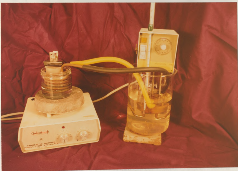
Figure 4.10 The system for protein adsorption measurement
