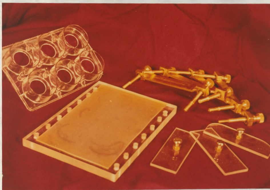
Figure 4.6 Modified 6 well incubation test cell
