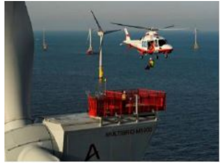
(b) Helicopter accessing top of turbine
