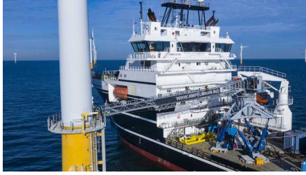
(a) Gangway access to top of transition piece
