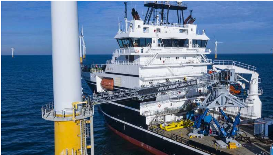
Figure 1.6: Photograph of an Ampelmann motion compensated gangway
