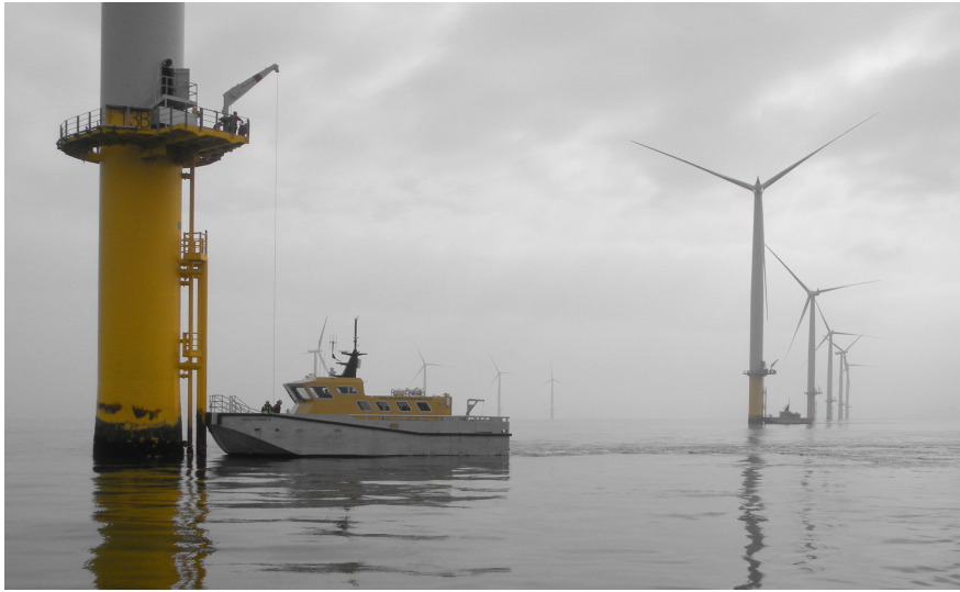
Figure 1.5: Photograph of a CTV at a turbine in calm seas
