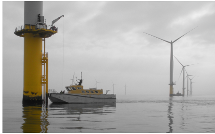
(c) CTV accessing boat landing point
