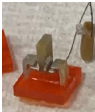
Figure 4.13: Picture of a sensor painted with silver paint.
