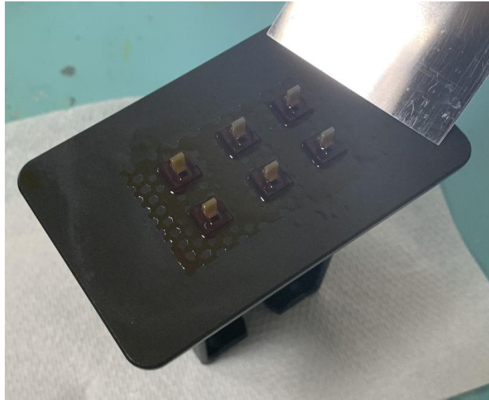
Figure 3.13: Build platform with printed objects, in the upper-right the metal scraper used to remove the models can be seen.
