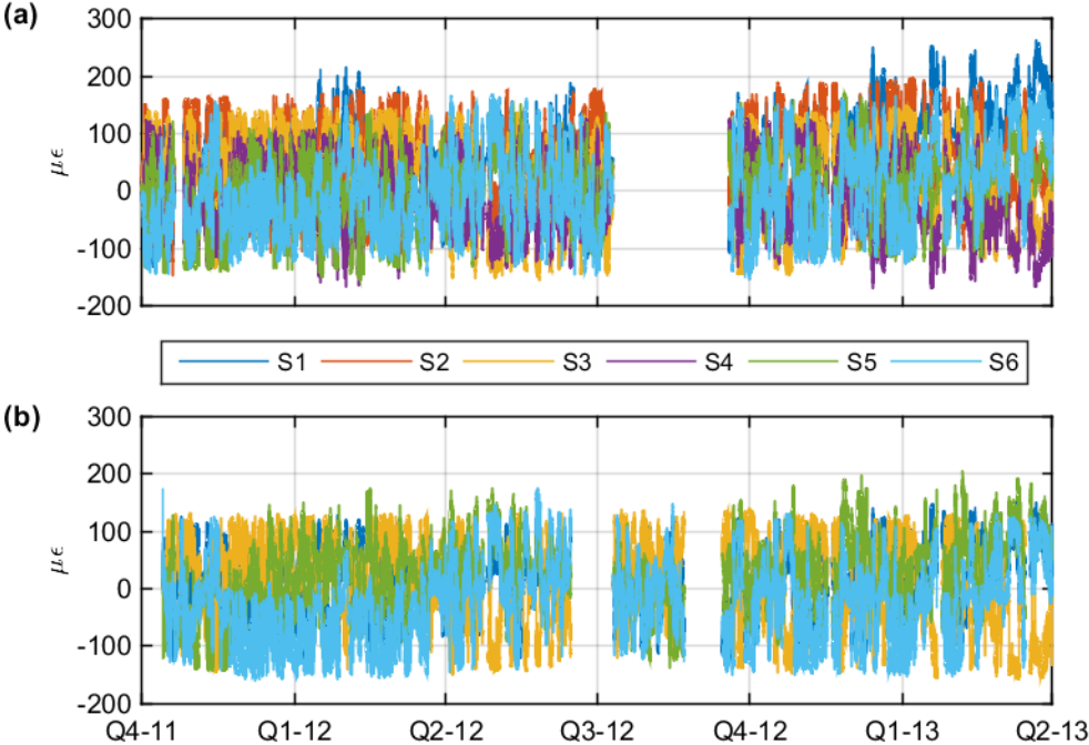
Figure 3-5. Ten minute average strain values, filtered to remove erroneous readings. (a) K1 global gauges S1-SGA to S6-SGA. (b) H4 global gauges S1-SGA, S3-SGA, S5-SGA, and S6-SGA.
