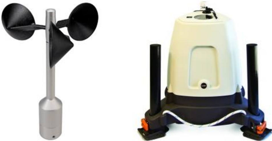
Figure 2-3. Wind speed measurement instruments. Left; cup anemometer (image from [43]). Right; LIDAR (image from [44]).
