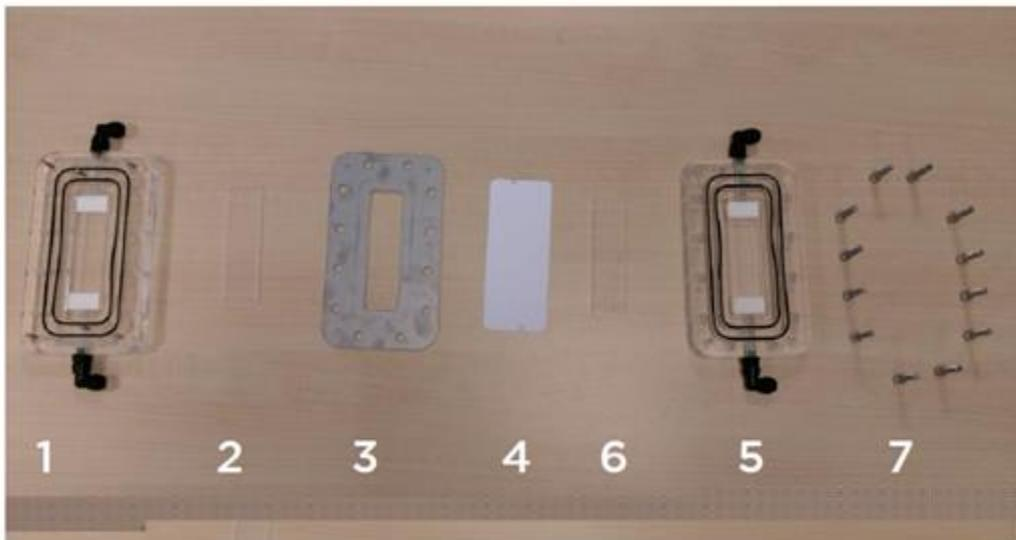
Figure 3.3. Components of the DCMD Membrane Module Configuration
