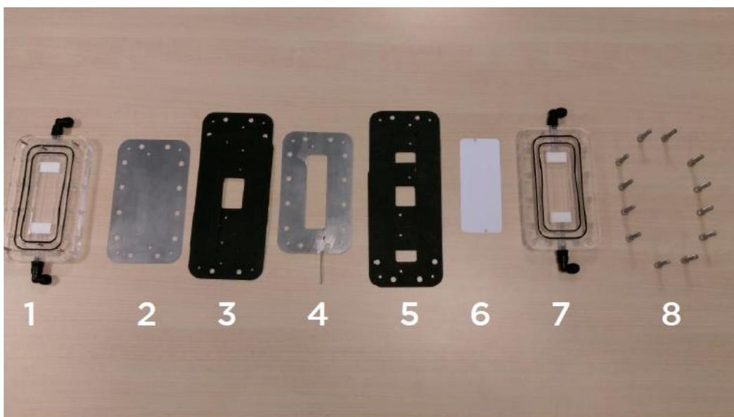
Figure 3.4. Components of the AGMD Membrane Module Configuration
