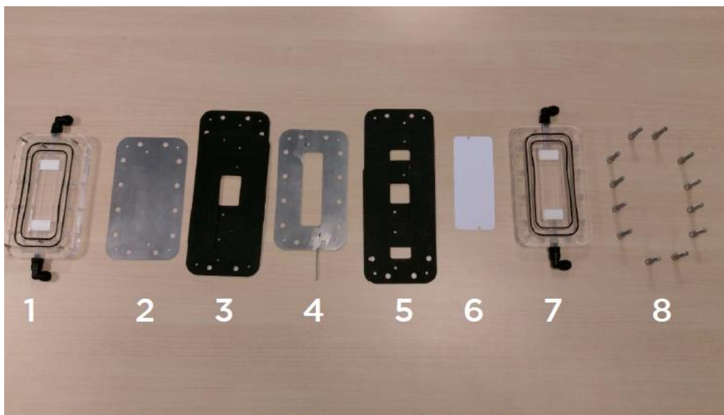
Figure 3.4. Components of the AGMD Membrane Module Configuration
