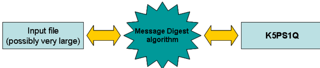
Figure 2.3 The Message Digest process (adapted from: (Menezes et al., 2001))
