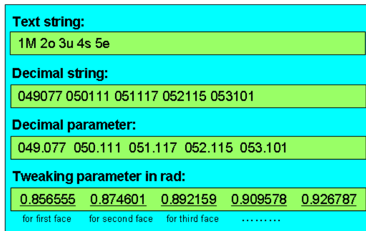
Figure 7.9 Information conversion and encoding for robust watermarking
