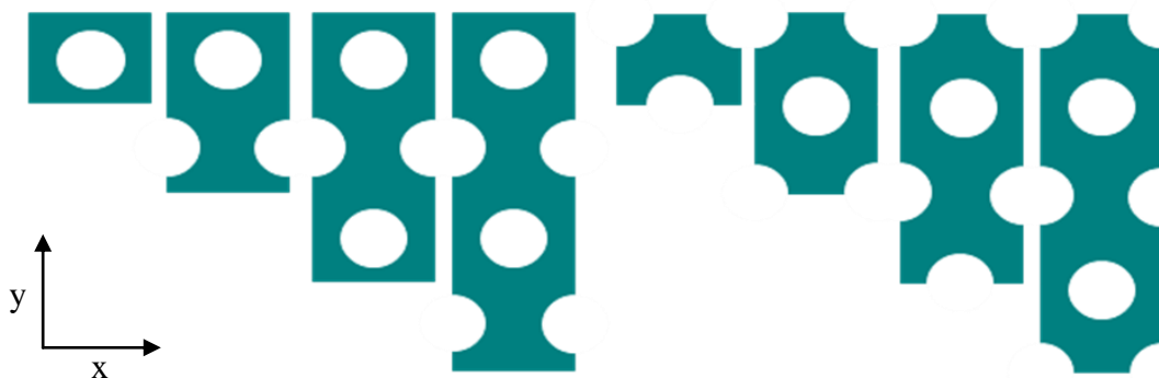
Figure 23 – Examples of beam cross sections for beams with and without surface perforations for 3D simulations
