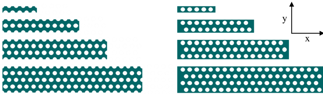
Figure 8 - Beams with and without surface perforations with constant length to depth aspect ratio and varying depths
