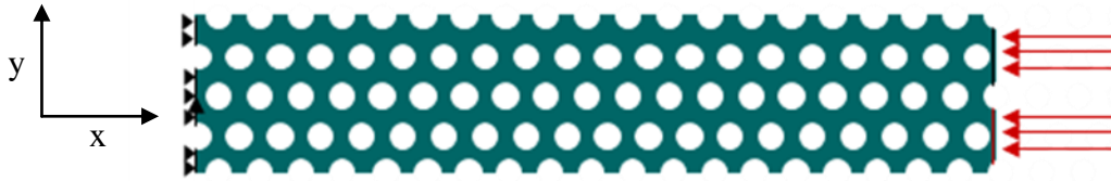
Figure 7 - Axial loading in the x-direction: horizontally fixed at the left end with the central node pinned in the y-direction on the left end and a uniform pressure applied at the free end.
