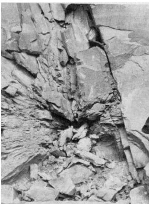
**Figure 5.24:** Photograph showing radial fractures emanating from blasting terminated by the presence of a natural fracture already existing in the rock. From Gretener 1983.
