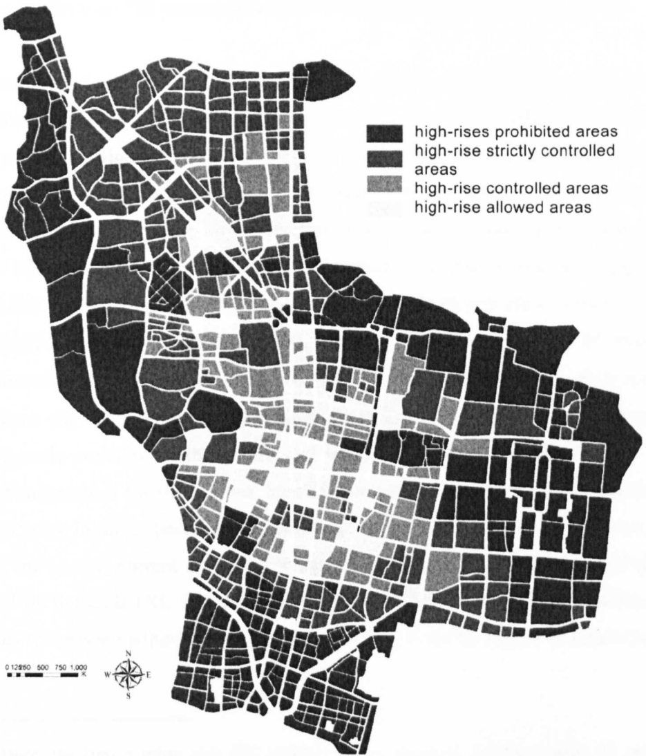
Figure 11.10 The height control of buildings in the old city as shown in the urban plan X (Wang, 2006, p53)
