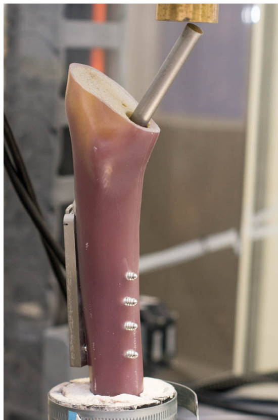
Figure 9.1: MISHS test setup for first specimen with head removed.
