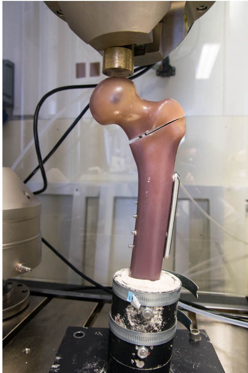
Figure 5.24: Fractured femur test setup.
