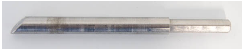
Figure 5.11: Original pin used to load SHS in femoral shaft test.
