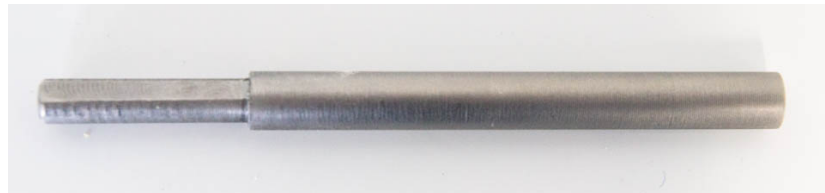
Figure 5.12: Modified pin used to load SHS in femoral shaft test.
