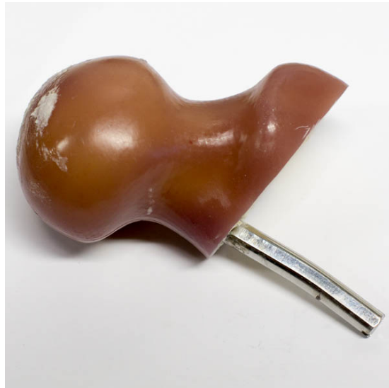
Figure 9.8: Plastic deformation of neck screw during fatigue test.
