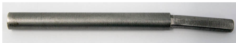
Figure 5.14: Deformed test pin after initial tests.
