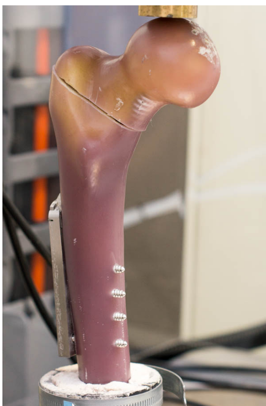
Figure 9.2: MISHS test setup for fractured femur.
