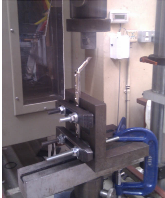
Figure 5.1: Setup for mechanical testing of the Synthes SHS.
