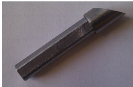
Figure 5.2: Test pin used to apply load to the SHS.
