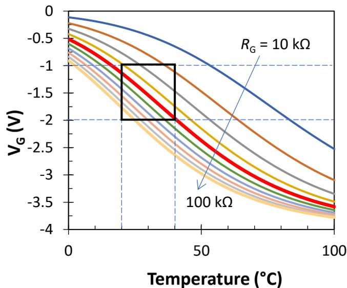
**Figure 6.4:** Effects of resistor  $R_G$  ( $10$  k to  $100$   $\text{k}\Omega$ ) on  $V_G$  as a function of temperature. The desirable temperature and voltage range for  $V_G$  are indicated by the black rectangle. The red thick curve corresponds to  $R_G = 50$   $\text{k}\Omega$ . The results correspond to  $V_{\text{IN}} = -4$  V.
