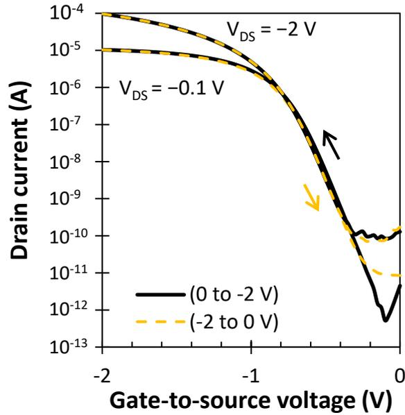
**Figure 3.10:** OTFT hysteresis measurement, forward ( $V_{GS} = 0$  to  $-2$  V) and reverse ( $V_{GS} = -2$  to  $0$  V) sweep (arrows show the direction of sweep) in linear ( $V_{DS} = -0.1$  V) and saturation ( $V_{DS} = -2$  V) regimes.
