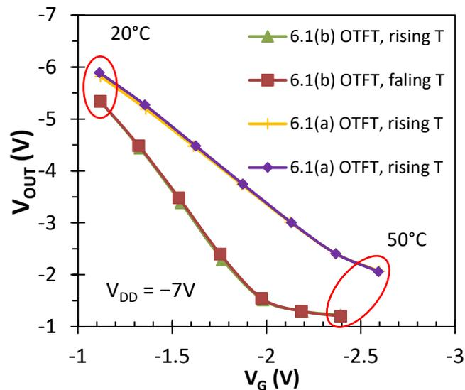
**Figure 6.9:** Repeated measurements of  $V_{\text{OUT}}$  as a function of  $V_{\text{G}}$  for  $V_{\text{IN}} = -4 \text{ V}$ ,  $V_{\text{DD}} = -7 \text{ V}$ ,  $R_{\text{D}} = 47 \text{ k}\Omega$ ,  $R_{\text{G}} = 50 \text{ k}\Omega$  and OTFTs of Figure 6.2(a) and (b). Rising and falling T represent ramping temperature from 20 to  $50^\circ\text{C}$  and from 50 to  $20^\circ\text{C}$  respectively.
