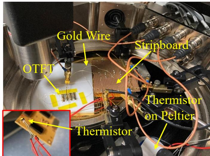
**Figure 3.15:** Temperature sensor measurement setup
