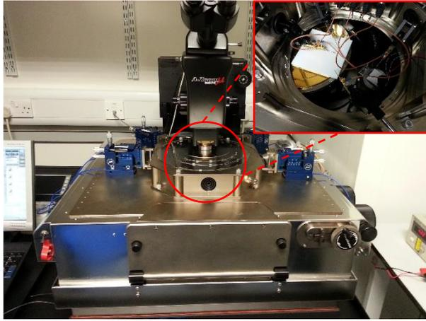
**Figure 3.3:** Agilent B1500A and probe station for device characterisation.
