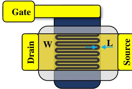
**Figure 3.12:** Top view of an organic thin-film transistor with interdigitated source/drain contacts.
