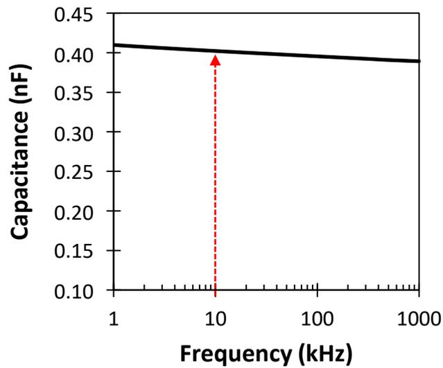
**Figure 3.4:** MIM capacitance as a function of AC frequency.
