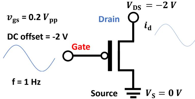
**Figure 3.11:** AC transconductance measurement setup.
