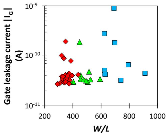
**Figure 4.19:** Gate leakage current as a function of  $W/L$  for wide-gate OTFTs with interdigitated source/drain contacts and  $L = 20$  to  $30 \mu\text{m}$  (square),  $L = 30$  to  $40 \mu\text{m}$  (triangles), or  $L = 40$  to  $50 \mu\text{m}$  (diamonds).
