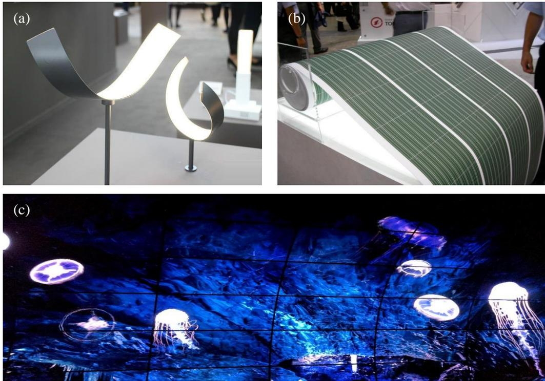
**Figure 1.1:** OLED ultra-thin panel for lighting [1.13] (a), large area printed organic photovoltaic [1.14] (b), and flexible display [1.15] (c)
