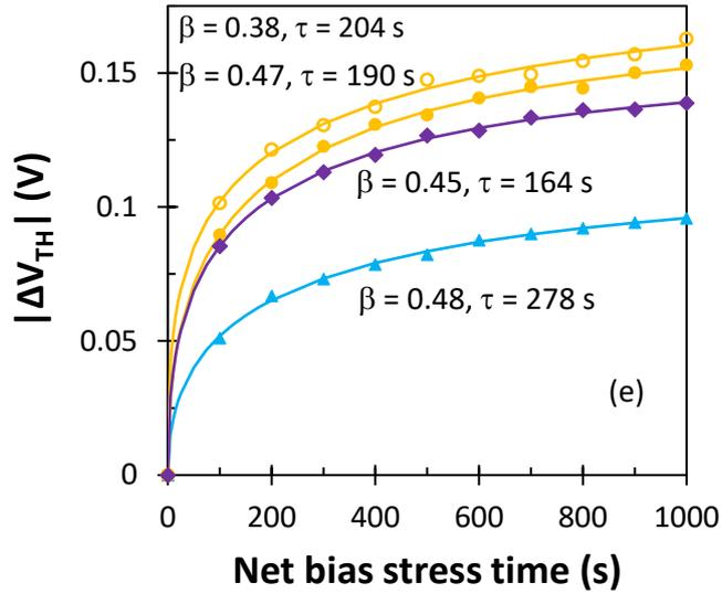
**Figure 5.9:** Threshold voltage shift of 5-6 months aged OTFTs as a function of net bias stress time. The legend of Fig. 5.8 applies.
