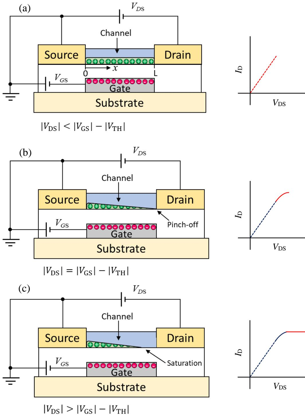
**Figure 2.3:** OTFT channel formation. Linear regime ( $|V_{DS}| < |V_{GS}| - |V_{TH}|$ ) (a), pinch-off ( $|V_{DS}| = |V_{GS}| - |V_{TH}|$ ) (b), and saturation regime ( $|V_{DS}| > |V_{GS}| - |V_{TH}|$ ) (c).
