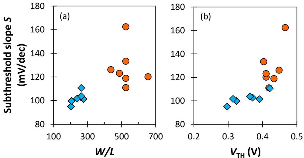
**Figure 4.11:** Subthreshold slope as a function of  $W/L$  (a) and  $V_{TH}$  (b) for narrow-gate OTFTs with interdigitated source/drain contacts and  $L < 10 \mu\text{m}$  (circles) or  $L = 10$  to  $20 \mu\text{m}$  (diamonds).
