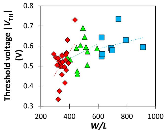
**Figure 4.15:** Threshold voltage as a function of  $W/L$  for wide-gate OTFTs with interdigitated source/drain contacts and  $L = 20$  to  $30 \mu\text{m}$  (square),  $L = 30$  to  $40 \mu\text{m}$  (triangles), or  $L = 40$  to  $50 \mu\text{m}$  (diamonds).
