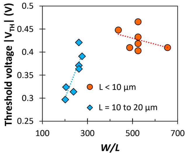
**Figure 4.6:** Threshold voltage as a function of  $W/L$  for narrow-gate OTFTs with interdigitated source/drain contacts and  $L < 10 \mu\text{m}$  (circles) or  $L = 10$  to  $20 \mu\text{m}$  (diamonds).
