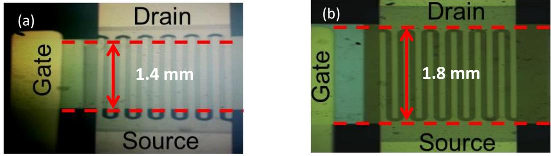
**Figure 4.13:** Gate width manipulation in wide-gate OTFTs resulting in reduced gate width of 1.4 mm and  $W = 15.40$  mm (a) and full gate width of 1.8 mm and  $W = 18.23$  mm (b). Dashed horizontal lines show the gate width boundaries.
