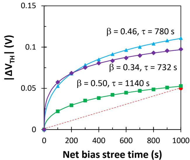
**Figure 5.6:** Threshold voltage shift of freshly fabricated OTFTs as a function of net bias stress time. The legend of Fig. 5.5 applies.
