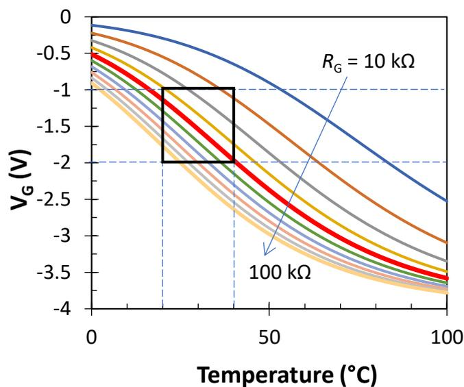
**Figure 6.4:** Effects of resistor  $R_G$  ( $10$  k to  $100$  k $\Omega$ ) on  $V_G$  as a function of temperature. The desirable temperature and voltage range for  $V_G$  are indicated by the black rectangle. The red thick curve corresponds to  $R_G = 50$  k $\Omega$ . The results correspond to  $V_{IN} = -4$  V.
