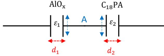
**Figure 3.5:** Gate dielectric bi-layer, where  $A$  is the contact area (identical for  $\text{AlO}_x$  and  $\text{C}_{18}\text{PA}$ ),  $\epsilon_1$ ,  $\epsilon_2$  and  $d_1$ ,  $d_2$  are the permittivity and thicknesses of  $\text{AlO}_x$  and  $\text{C}_{18}\text{PA}$  respectively.
