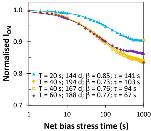
**Figure 5.8:** Normalised on-state drain current of 5-6 months aged OTFTs as a function of net bias stress time.
