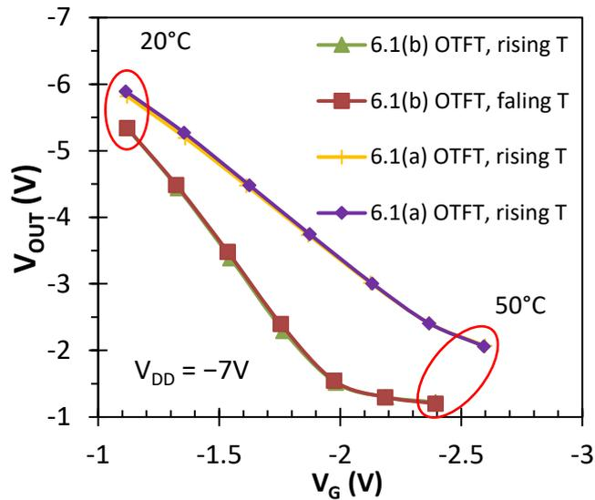
**Figure 6.9:** Repeated measurements of  $V_{\text{OUT}}$  as a function of  $V_G$  for  $V_{\text{IN}} = -4 \text{ V}$ ,  $V_{\text{DD}} = -7 \text{ V}$ ,  $R_{\text{D}} = 47 \text{ k}\Omega$ ,  $R_{\text{G}} = 50 \text{ k}\Omega$  and OTFTs of Figure 6.2(a) and (b). Rising and falling T represent ramping temperature from 20 to 50°C and from 50 to 20°C respectively.
