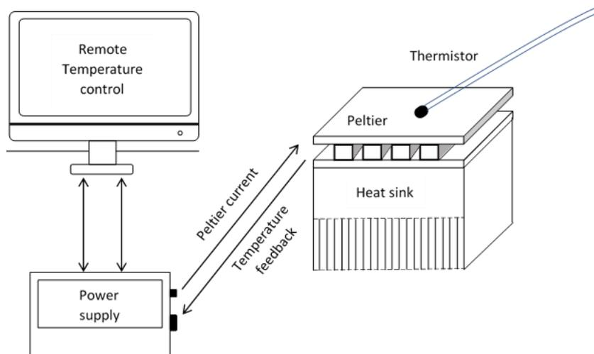
**Figure 3.16:** Thermistor temperature control system setup.
