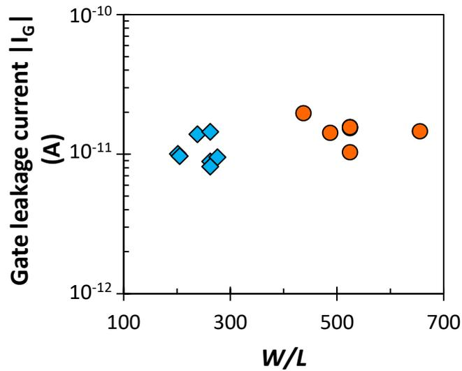
**Figure 4.12:** Gate leakage current as a function of  $W/L$  for narrow-gate OTFTs with interdigitated source/drain contacts and  $L < 10 \mu\text{m}$  (circles) or  $L = 10$  to  $20 \mu\text{m}$  (diamonds).
