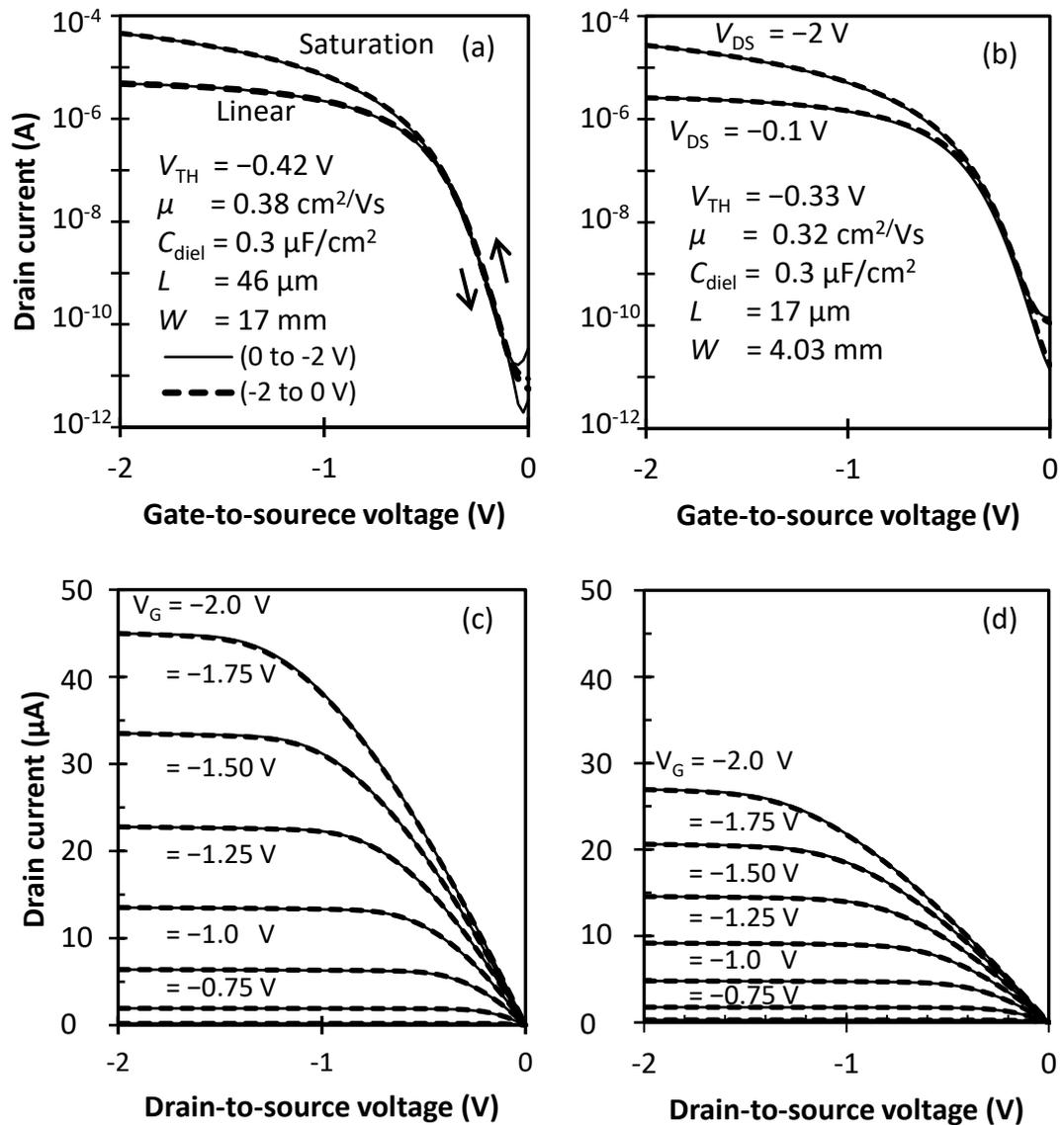
**Figure 4.4:** Transfer (a, b) and output (c, d) characteristics for wide-gate (a, c) and narrow-gate (b, d) OTFTs on PEN. Each curve shows hysteresis measurement from 0 to -2 V (solid line) and back (dash lines).
