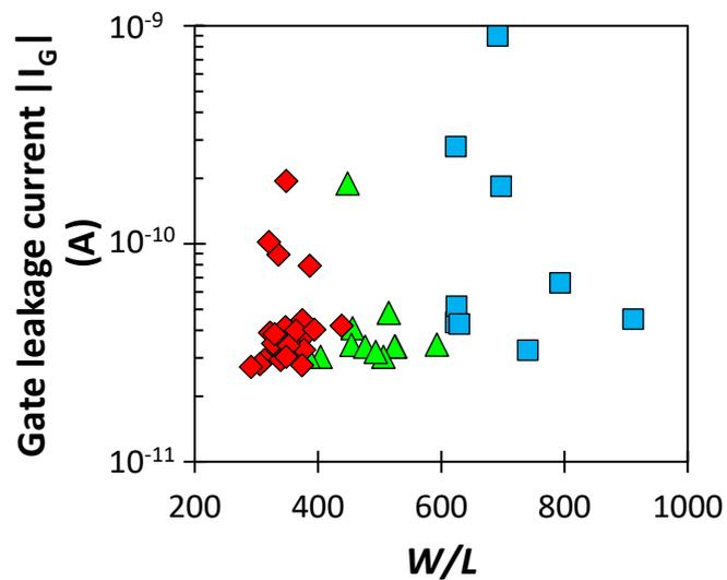
**Figure 4.19:** Gate leakage current as a function of  $W/L$  for wide-gate OTFTs with interdigitated source/drain contacts and  $L = 20$  to  $30 \mu\text{m}$  (square),  $L = 30$  to  $40 \mu\text{m}$  (triangles), or  $L = 40$  to  $50 \mu\text{m}$  (diamonds).
