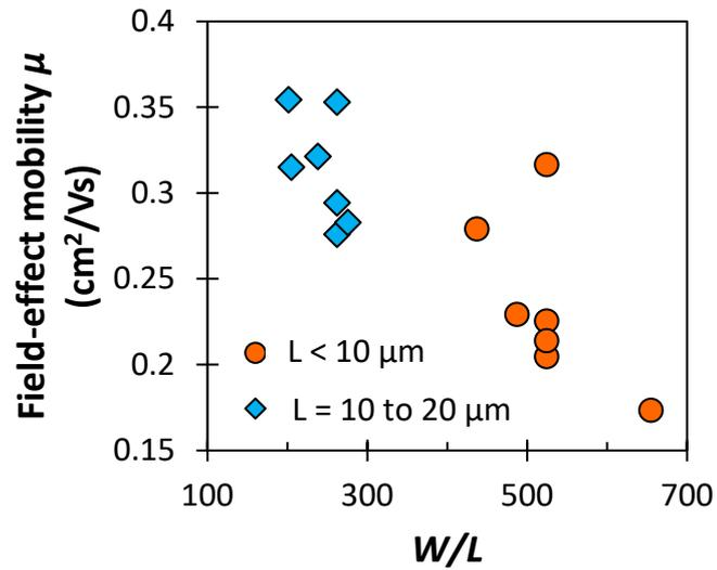
**Figure 4.5:** Field-effect mobility as a function of  $W/L$  for narrow-gate OTFTs with interdigitated source/drain contacts and  $L < 10 \mu\text{m}$  (circles) or  $L = 10$  to  $20 \mu\text{m}$  (diamonds).
