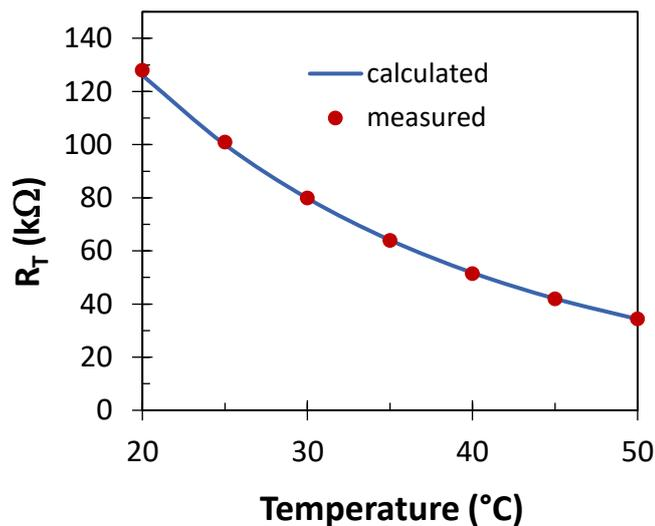
**Figure 6.3:** Temperature response of a thermistor having a nominal resistance of 100 kΩ at 25°C.
