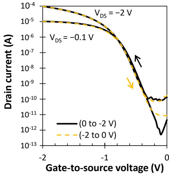
**Figure 3.10:** OTFT hysteresis measurement, forward ( $V_{GS} = 0$  to  $-2$  V) and reverse ( $V_{GS} = -2$  to  $0$  V) sweep (arrows show the direction of sweep) in linear ( $V_{DS} = -0.1$  V) and saturation ( $V_{DS} = -2$  V) regimes.
