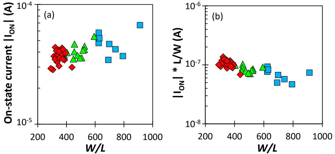
**Figure 4.16:** On-state drain current (a) and normalised on-state drain current (b) as functions of  $W/L$  and channel lengths  $L = 20$  to  $30 \mu\text{m}$  (squares),  $30$  to  $40 \mu\text{m}$  (triangles) and  $40$  to  $50 \mu\text{m}$  (diamonds).
