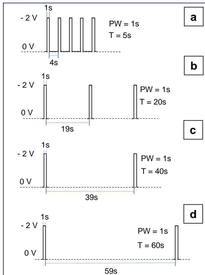
**Figure 5.1:** AC pulse signals with 1-s-pulse width (PW), on-state and off-state voltages of  $-2$  V and  $0$  V, and period ( $T$ ) of 5s (a), 20s (b), 40s (c) and 60s (d). During the bias stress the same pulse was applied to the gate and drain of the transistor.
