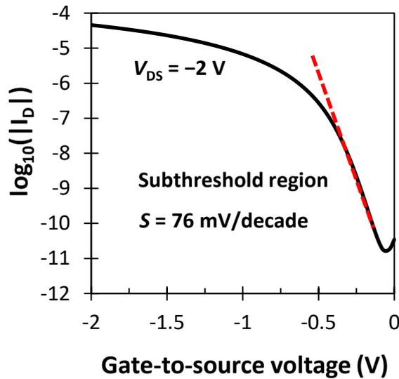
**Figure 3.8:** Subthreshold slope extraction from the subthreshold region.
