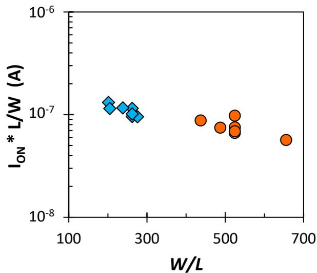
**Figure 4.8:** Normalised on-state drain current as a function of  $W/L$  for narrow-gate OTFTs with interdigitated source/drain contacts and  $L < 10 \mu\text{m}$  (circles) and  $L = 10$  to  $20 \mu\text{m}$  (diamonds).
