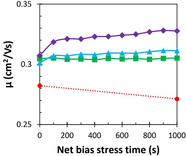
**Figure 5.4:** Field-effect mobility  $\mu$  as a function of net bias stress time. The legend of Fig. 5.2 applies.
