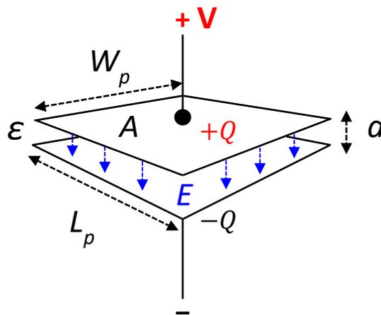
**Figure 2.1:** Schematic diagram of MIM structure.
