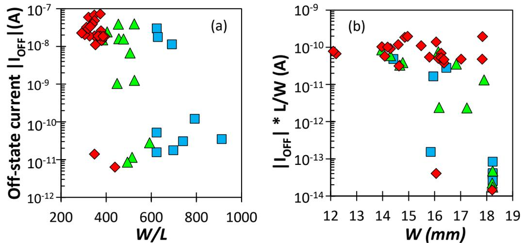
**Figure 4.17:** Off-state drain current (a) and normalised off-state drain current (b) as functions of  $W/L$  and width  $W$  respectively, for channel length  $L = 20$  to  $30 \mu\text{m}$  (squares),  $30$  to  $40 \mu\text{m}$  (triangles) and  $40$  to  $50 \mu\text{m}$  (diamonds).
