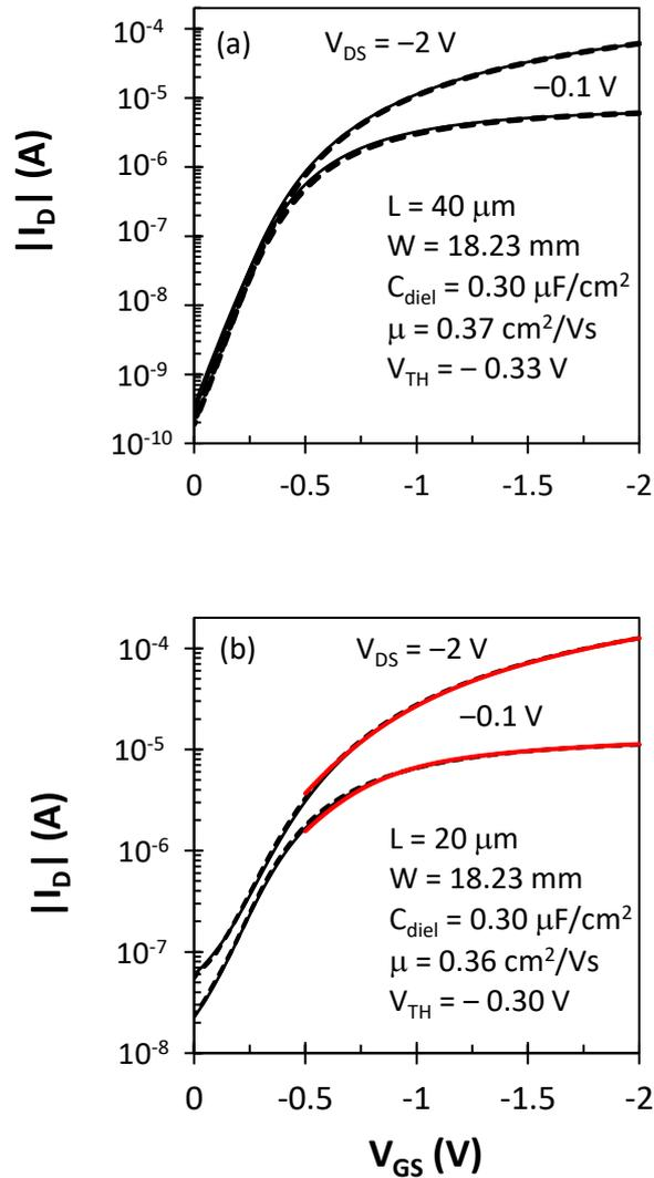
**Figure 6.2:** Transfer characteristics of OTFTs used in the temperature sensor and verification model. Solid black lines and dotted lines represent hysteresis for  $V_{GS}$  ramped in forward direction (0 to  $-2$  V) and reverse ( $-2$  to 0 V) respectively. Solid red lines represents the transistor model.
