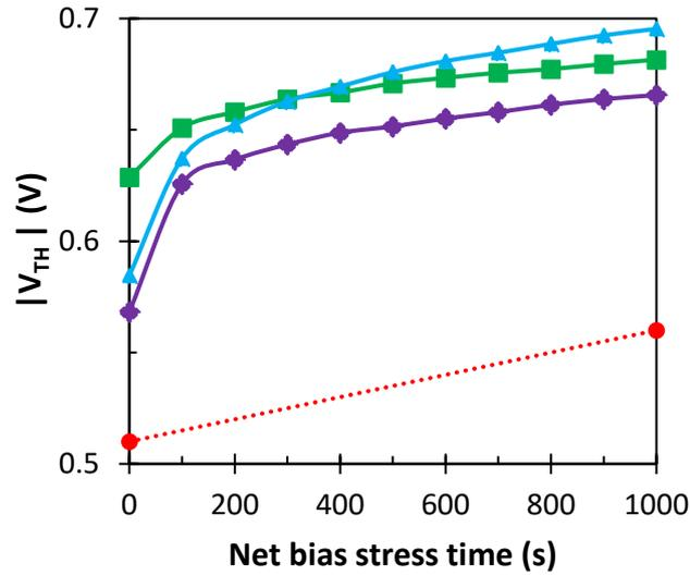
**Figure 5.3:** Threshold voltage  $V_{TH}$  as a function of net bias stress time. The legend of Figure 5.2 applies.
