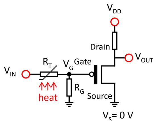
**Figure 3.14:** OTFT-based temperature sensor schematic.
