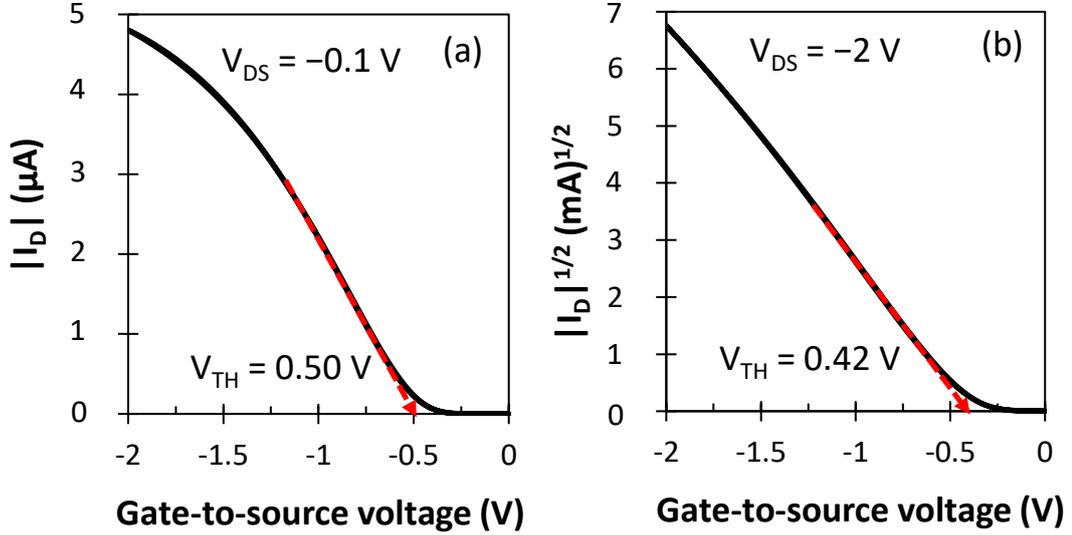
**Figure 3.7:** Threshold voltage extraction from slopes of  $I_D$  and  $\sqrt{I_D}$  as functions of  $V_{GS}$  in linear ( $V_{DS} = -0.1$  V) (a) and saturation ( $V_{DS} = -2$  V) (b) regimes.
