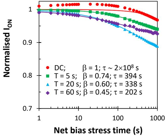
**Figure 5.5:** Normalised on-state drain current of freshly fabricated OTFTs as a function of net bias stress time. Points (symbols) represent measured data and lines are the stretched exponential fits with fitting parameters of  $\beta$  and  $\tau$ .
