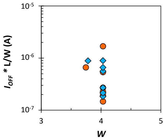
**Figure 4.10:** Normalised off-state drain current as a function of  $W$  for narrow-gate OTFTs with interdigitated source/drain contacts and  $L < 10 \mu\text{m}$  (circles) or  $L = 10$  to  $20 \mu\text{m}$  (diamonds).
