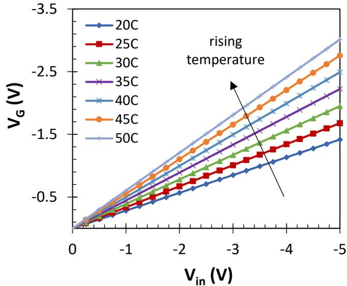
**Figure 6.5:**  $V_G$  as a function of  $V_{IN}$  for temperatures ranging from 20 to 50°C and  $R_G = 50 \text{ k}\Omega$ .
