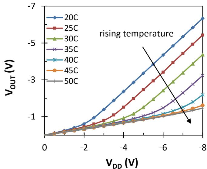
**Figure 6.7:**  $V_{OUT}$  as a function of  $V_{DD}$  for temperatures between 20 and 50°C,  $R_G = 50 \text{ k}\Omega$ ,  $R_D = 47 \text{ k}\Omega$  and  $V_{IN} = -4\text{V}$ .
