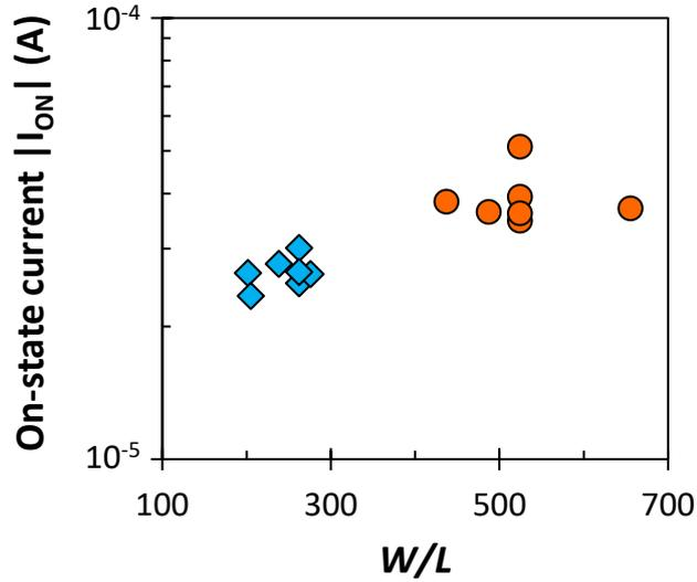
**Figure 4.7:** On-state drain current as a function of  $W/L$  for narrow-gate OTFTs with interdigitated source/drain contacts and  $L < 10 \mu\text{m}$  (circles) or  $L = 10$  to  $20 \mu\text{m}$  (diamonds).
