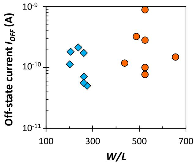
**Figure 4.9:** Off-state drain current as a function of  $W/L$  for narrow-gate OTFTs with interdigitated source/drain contacts and  $L < 10 \mu\text{m}$  (circles) or  $L = 10$  to  $20 \mu\text{m}$  (diamonds).
