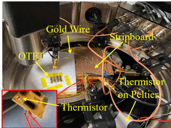
**Figure 3.15:** Temperature sensor measurement setup
