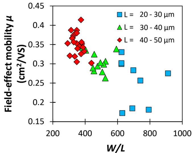
**Figure 4.14:** Field-effect mobility as a function of  $W/L$  for wide-gate OTFTs with interdigitated source/drain contacts and  $L = 20$  to  $30 \mu\text{m}$  (square),  $L = 30$  to  $40 \mu\text{m}$  (triangles), or  $L = 40$  to  $50 \mu\text{m}$  (diamonds).
