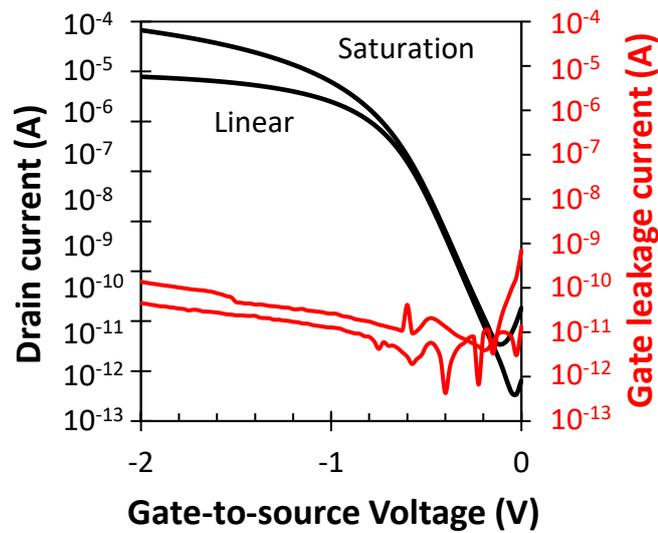
**Figure 3.6:** Transfer characteristics in linear ( $V_{DS} = -0.1$  V) and saturation regime ( $V_{DS} = -2$  V) for  $V_{GS}$  sweep from 0 to  $-2$  V.
