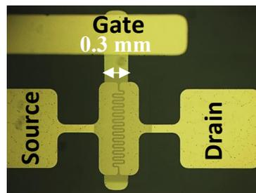
**Figure 4.3:** Top-view of narrow-gate width OTFT with  $L = 17 \mu m$  and  $W = 4.03 \text{ mm}$ .
