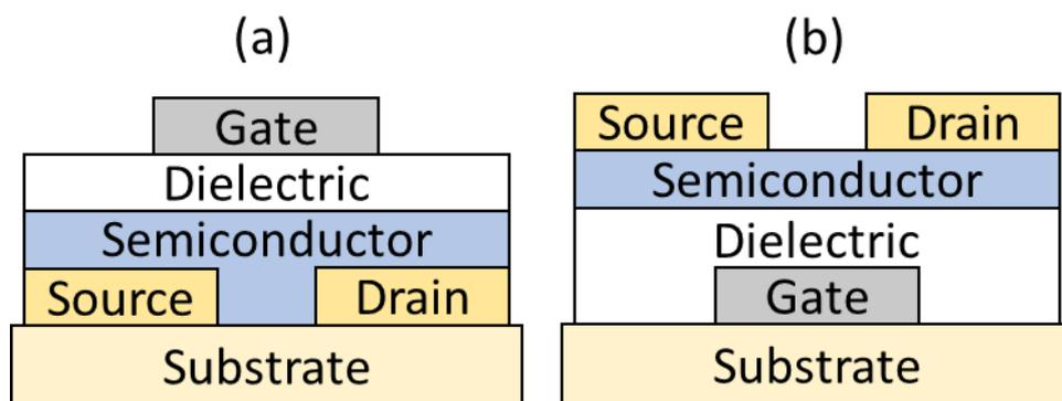
**Figure 2.2:** OTFT structures: TGBC (a) and BGTC (b).
