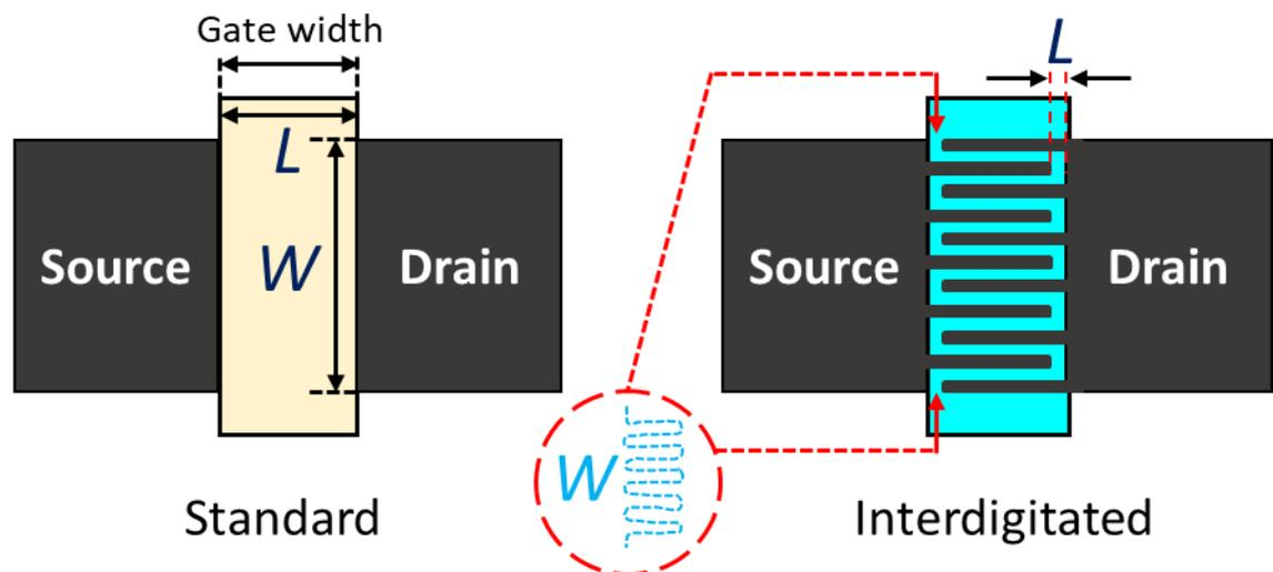
**Figure 4.1:** Standard rectangular and interdigitated source/drain contacts.
