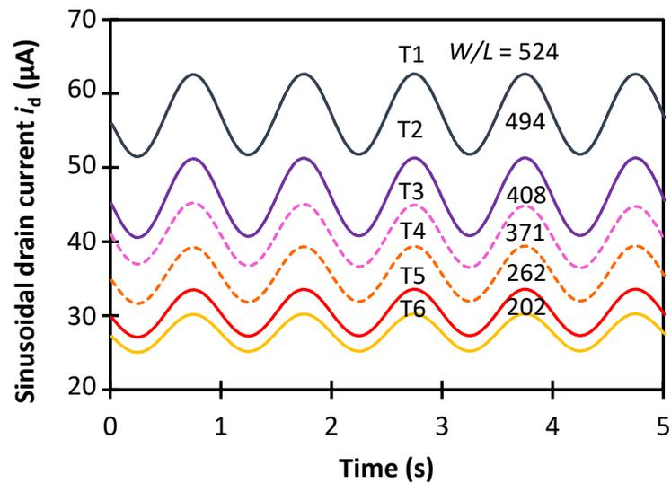
**Figure 4.20:** Sinusoidal drain current as a function of time (for  $v_{gs}$  of  $-0.2V_{pp}$ , and  $V_{DS}$  and  $V_S$  of  $-2\text{ V}$  and  $0\text{ V}$  respectively). The solid and dashed lines correspond to narrow- and wide-gate transistors, respectively.
