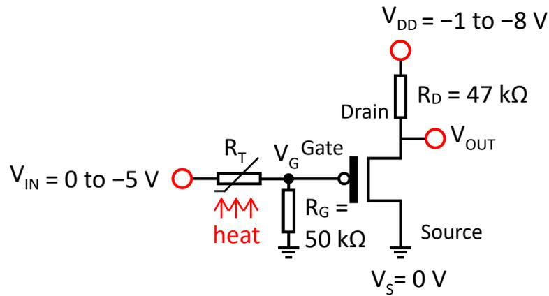
**Figure 6.1:** OTFT based temperature sensor.  $V_{IN} = 0$  to  $-5$  V,  $V_{DD} = -1$  to  $-8$  V,  $V_S = 0$  V.  $R_T$  has nominal resistance of  $100$  k $\Omega$  at  $25^\circ$  C and  $R_D = 47$  k $\Omega$ .
