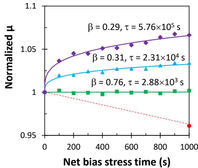
**Figure 5.7:** Normalised field-effect mobility of freshly fabricated OTFTs as a function of net bias stress time. The legend of Fig. 5.5 applies.
