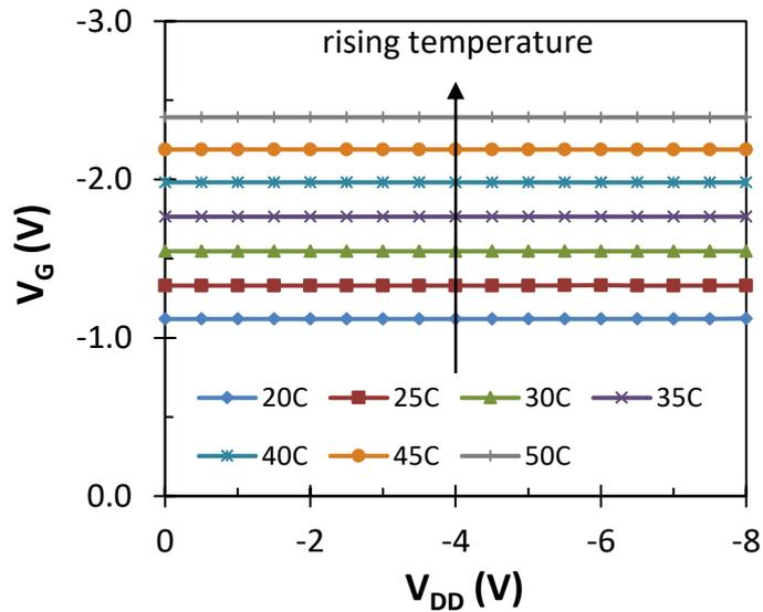
**Figure 6.6:** V<sub>G</sub> as a function of V<sub>DD</sub> for temperatures between 20 and 50°C,  $R_G = 50$  k $\Omega$ ,  $R_D = 47$  k $\Omega$  and  $V_{IN} = -4$  V. V<sub>G</sub> is referenced to ground.
