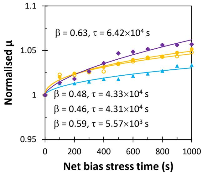
**Figure 5.10:** Normalised field-effect mobility of 5-6 months aged OTFTs as a function of net bias stress time. The legend of Fig. 5.8 applies.
