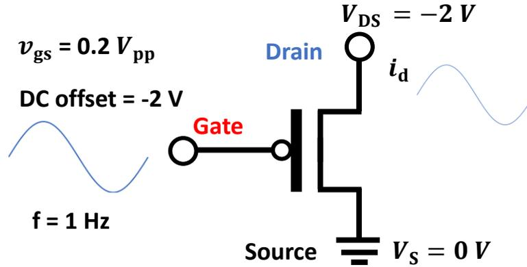
**Figure 3.11:** AC transconductance measurement setup.
