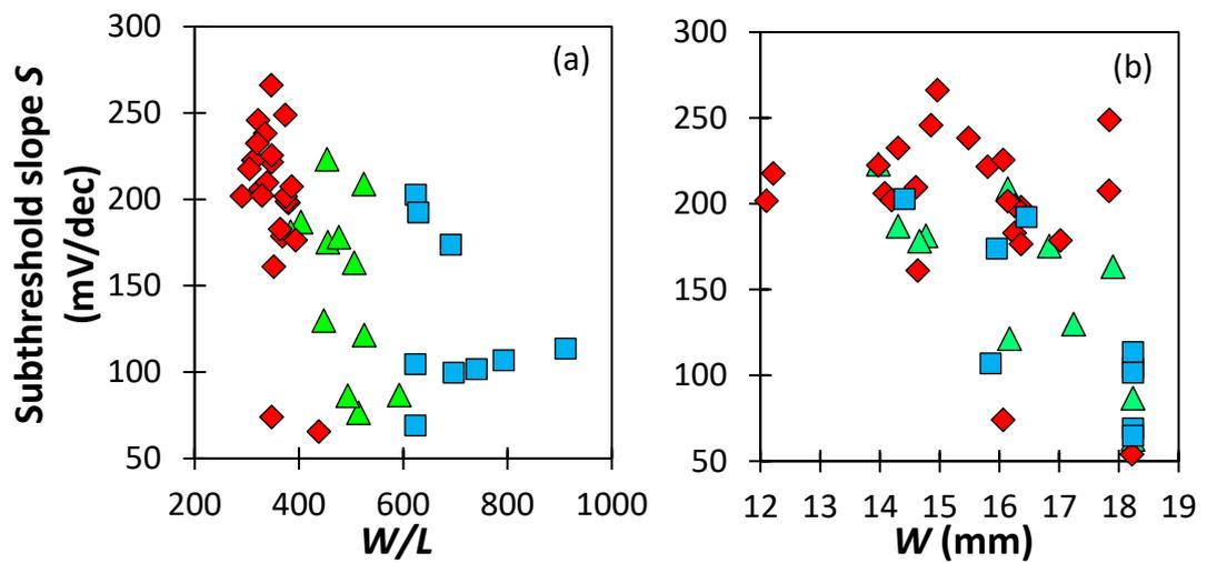
**Figure 4.18:** Subthreshold slope as a function of  $W/L$  (a) and  $W$  (b) for wide-gate OTFTs with interdigitated source/drain contacts and  $L = 20$  to  $30 \mu\text{m}$  (square),  $L = 30$  to  $40 \mu\text{m}$  (triangles), or  $L = 40$  to  $50 \mu\text{m}$  (diamonds).
