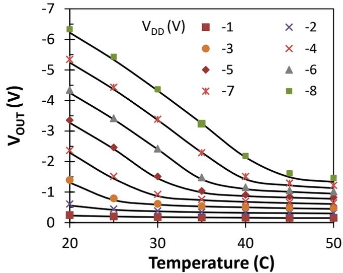
**Figure 6.8:**  $V_{OUT}$  of temperature sensor as a function of temperature between 20 and 50°C for  $R_G = 50 \text{ k}\Omega$ ,  $R_D = 47 \text{ k}\Omega$ , and  $V_{IN} = -4 \text{ V}$ . The solid black lines in (c) correspond to the sensor model.
