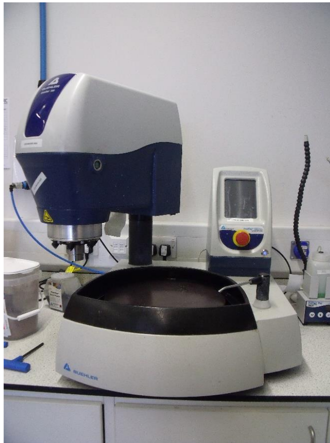
Figure 3.4 – EcoMet 300 Pro grinding/polishing machine
