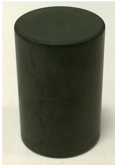
Figure 6.1 – Typical ATI 718Plus cylindrical test piece after heat treatment at 990°C for 180 minutes but prior to isothermal compression testing
