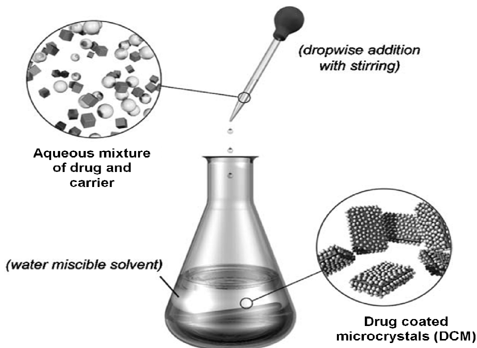
Figure 1.9 Process of preparing drug coated microcrystals (DCM) by dropping an aqueous mixture of drug and carrier in to a water miscible precipitating agent, modified from Murugesan et al (2005).
