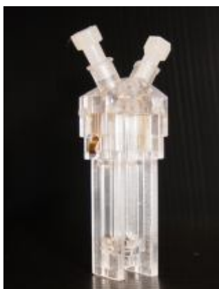
Figure 2.22 DTS 1060C- clear disposable zeta cell was used for zeta potential measurement.
