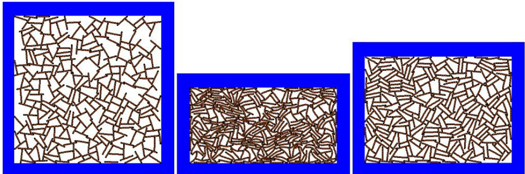
Figure B12. Effect of F_{range} during 1D compression and unloading (changing k_{Coul} )
