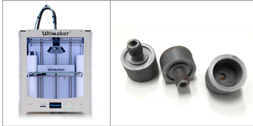
Figure A-3: Ultimaker 2 3D printer and 3D-printed PLA casings
