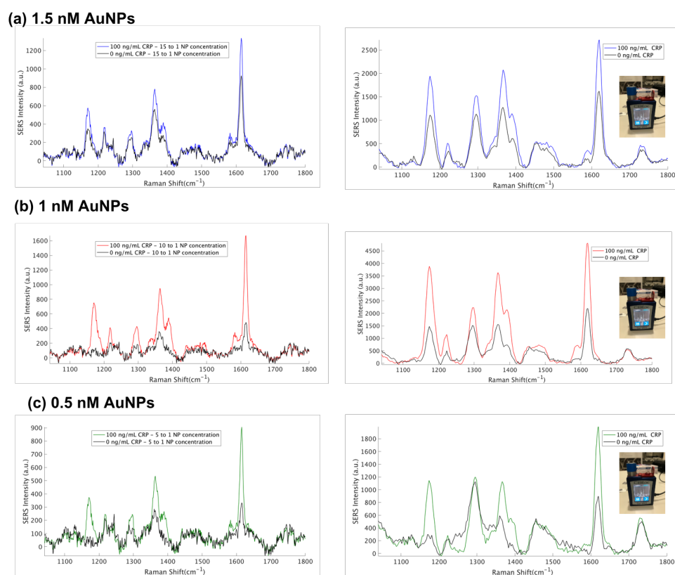
Figure 5.12: Corresponding average spectra from each SERS intensity map shown in figure 5.11 and handheld Raman analysis of each device - (a) 1.5 nM AuNP-Abs, a high SERS signal was observed for the control device relative to the sample device in both the SERS mapping and handheld analyses, (b) 1 nM AuNP-Abs, the best signal discrimination was observed at this concentration, with a lower SERS signal collected for the control but a higher signal collected for the sample compared with 1.5 nM AuNPs and (c) 0.5 nM AuNP-Abs, while signal discrimination was observed, the SERS intensity generated for both mapping and handheld analysis across all devices was low. Raman mapping analysis was performed at 633 nm laser excitation, 6s acquisition time, 0.73 mW laser power with a step size of 100 \mu\text{m} . Handheld Raman analysis was carried out at 638 nm laser wavelength, 0.2 s acquisition time and spectra were averaged from 3 scans.
