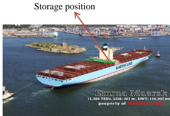
Figure 6-2: CO 2 container tank storage position.
