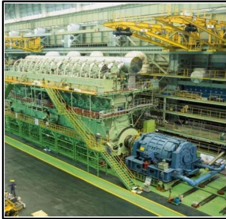
Figure 5-2: The Wärtsilä RT-flex96C Engine [42]
