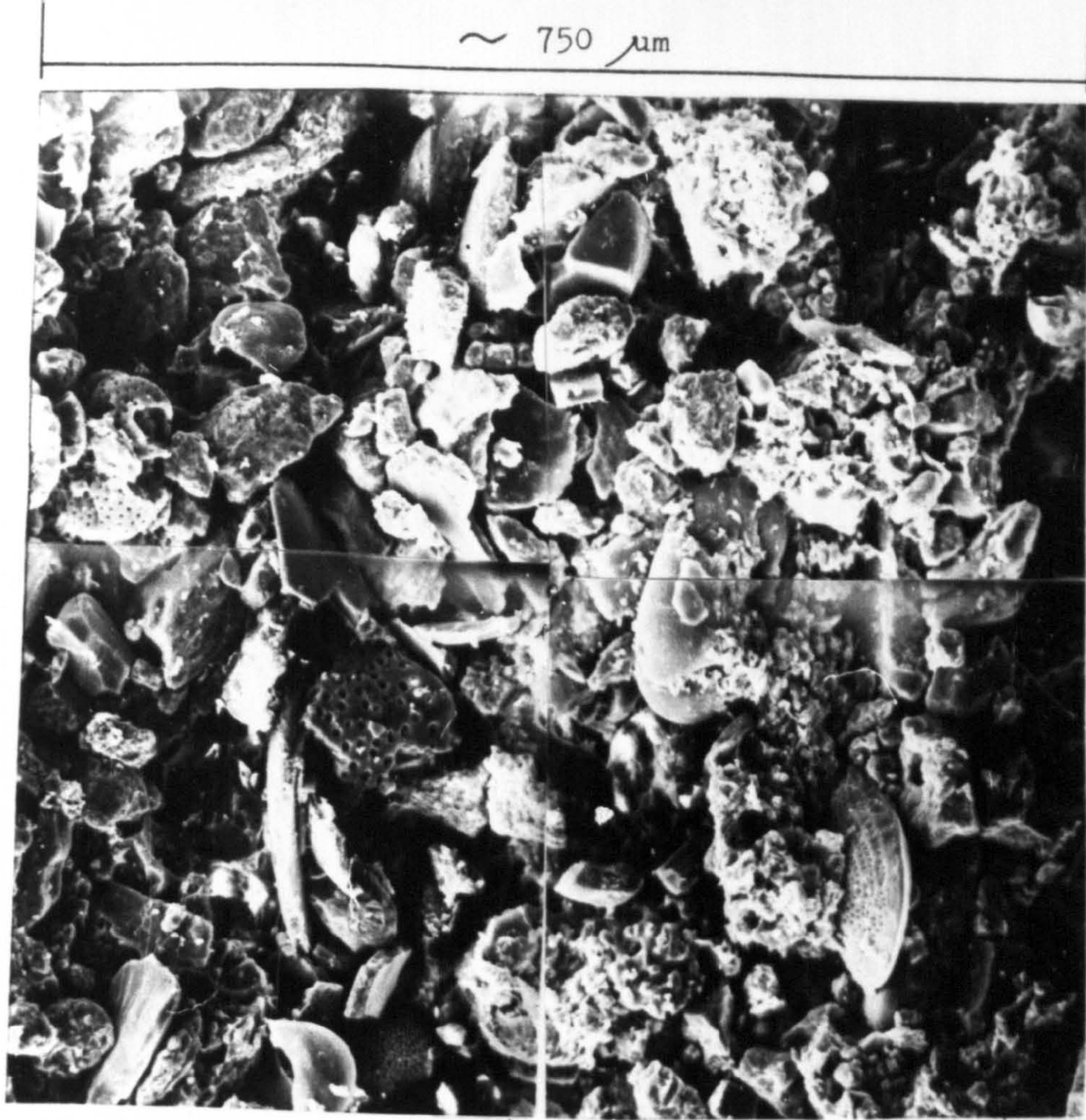
(e) Detailed view of composite microfabric x 160
