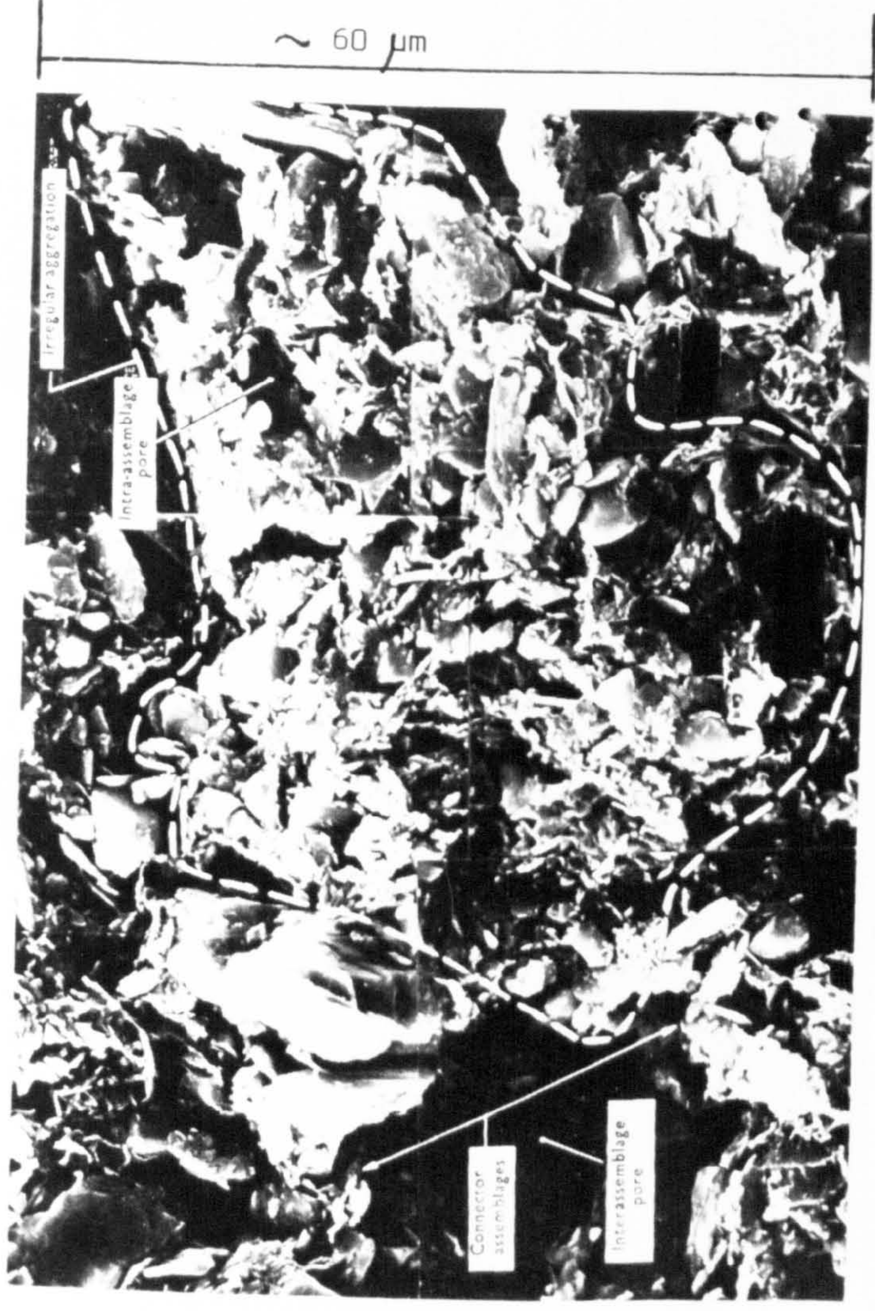
(b) Irregular aggregation with connector linkages x 1500
