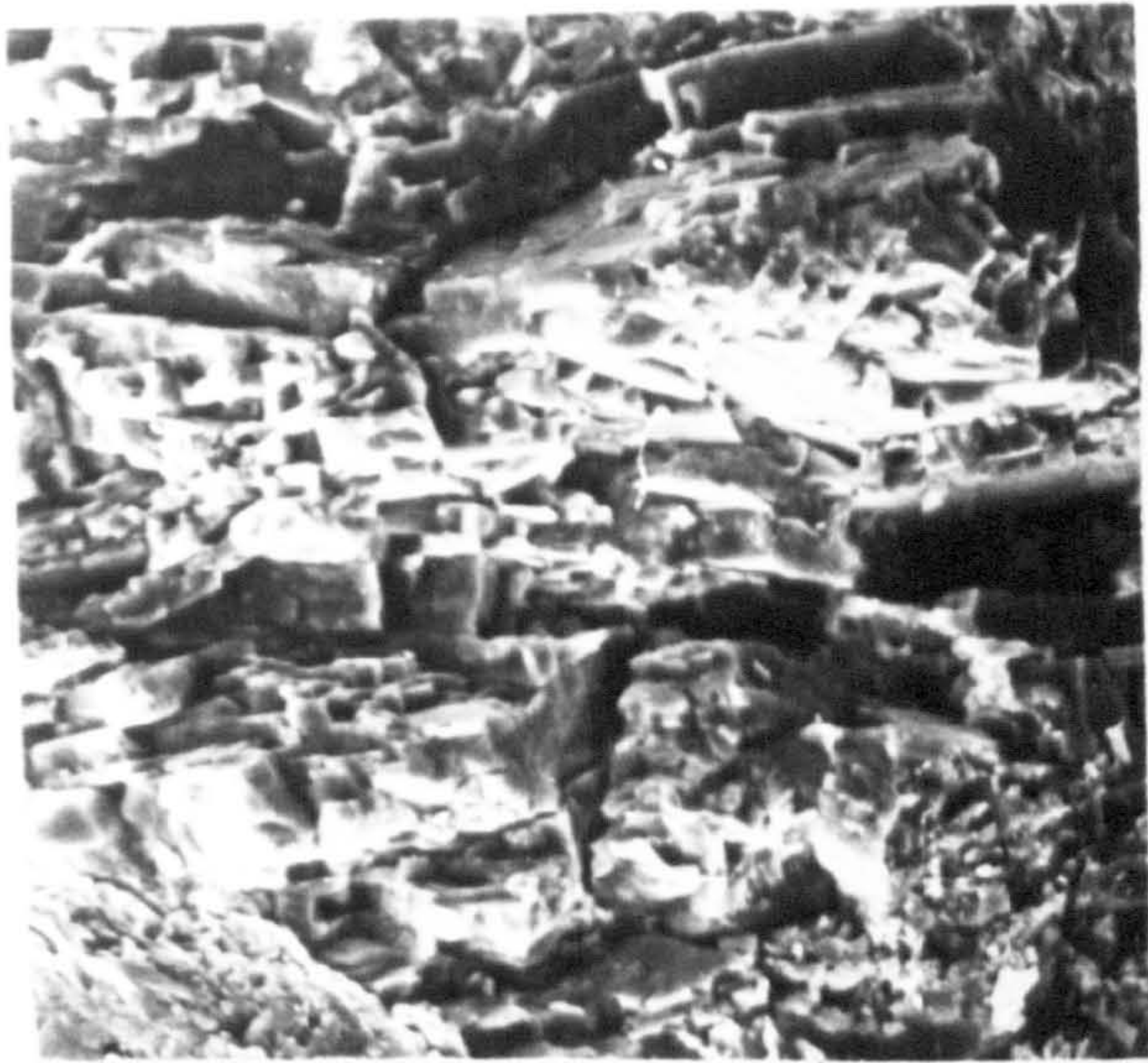
Sand Grains in State of Decomposition
