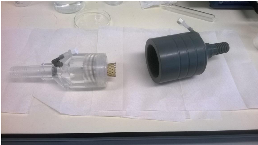
Figure 13: CoreValve placed in Pulse Duplicator.
