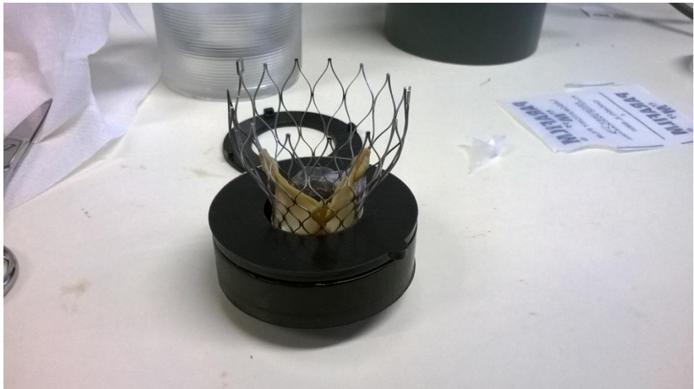
Figure 17: CoreValve placed onto Iris mechanism.
