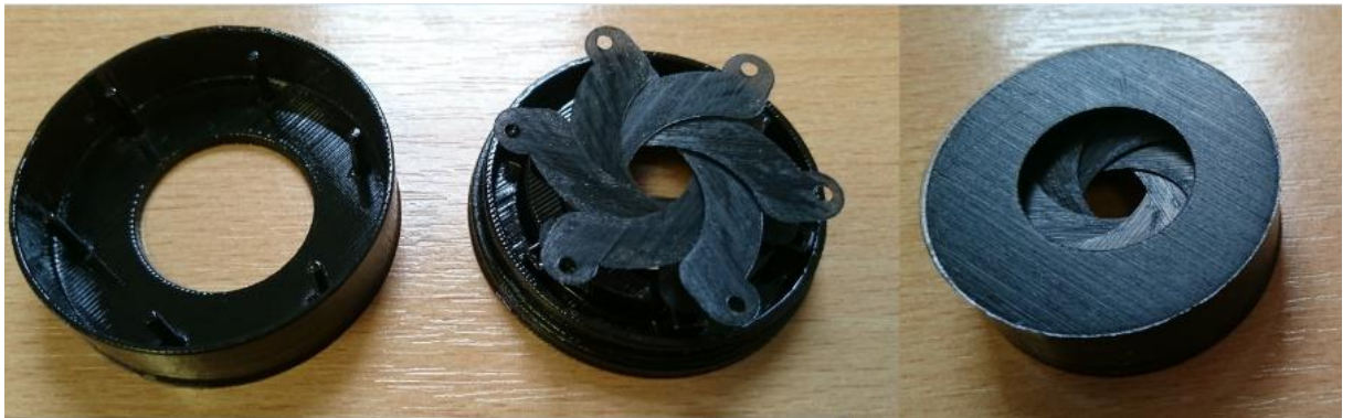
Figure 7: Iris mechanism idea, 3D printed parts.
