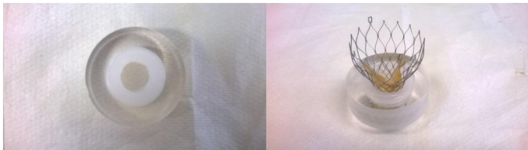
Figure 12: Valve attachment: (a) a holder with silicon mould, (b) the heart valve placed onto the holder.
