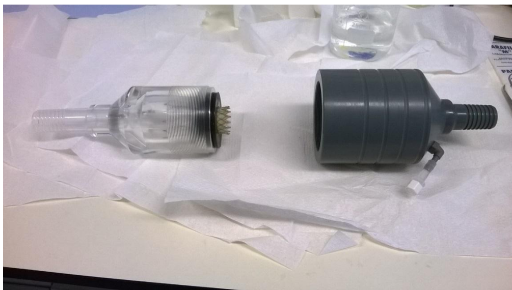
Figure 16: CoreValve placed onto Iris mechanism in Pulse Duplicator.
