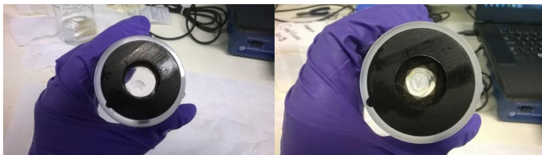
Figure 15: Iris mechanism placed in Pulse Duplicator: (a) bottom view 22 mm annulus, (b) bottom view 16 mm annulus.
