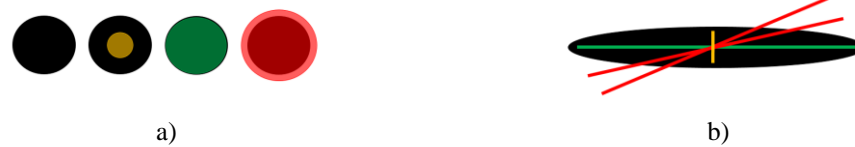
Figure 4.6: Examples of SE measurement where a) shows disk shape SE for radius measurement and b) linear SE for measuring orientation. In both cases black shapes are the original object, yellow are SE that fit comfortably thus don't describe the feature limits, green are SE the extrema that fits so describes feature properties well and red are SE that do not fit
