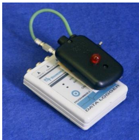
Figure 3.14 Portable data logger with 'event marker' system
