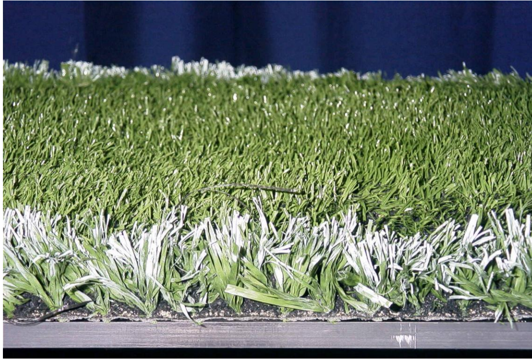
Figure.3.3 Turf (T3), with rubber and sand infill
