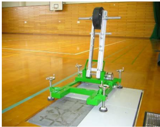
Figure 2.3 Prototype vertical impact test rig (Nunome et al, 2008)
