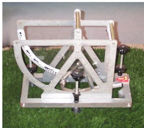
Figure 2.5 Modified Le Roux Pendulum
