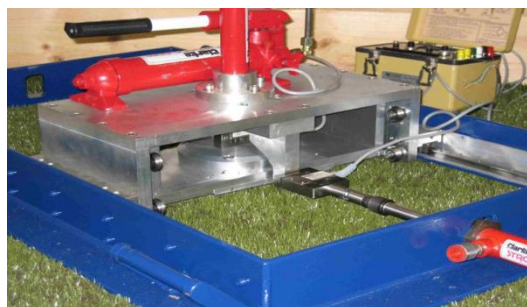
Figure 2.9 SERG sports surface traction rig
