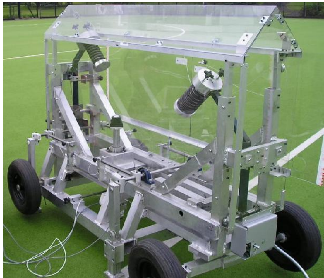
Figure 6.27 Strathclyde Sports Turf Testing Rig (SSTTR)
