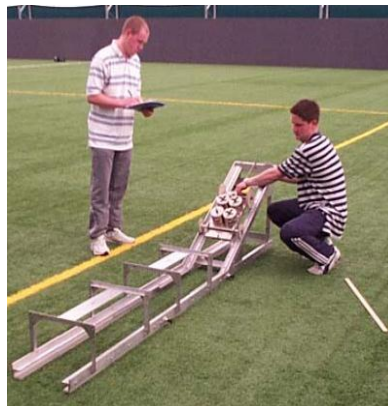
Figure 2.4 BS7044 Sliding distance test
