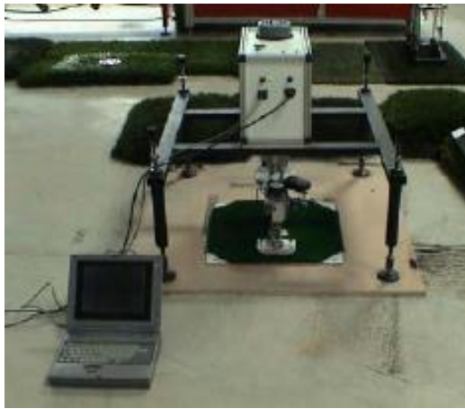
Figure 2.6 Securisport Sports Surface Tester
