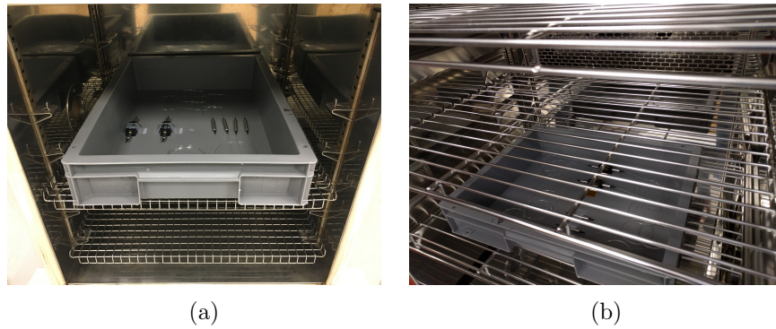
Figure 3.13: Parts placed in the (a) thermal & (b) humidity chamber.
