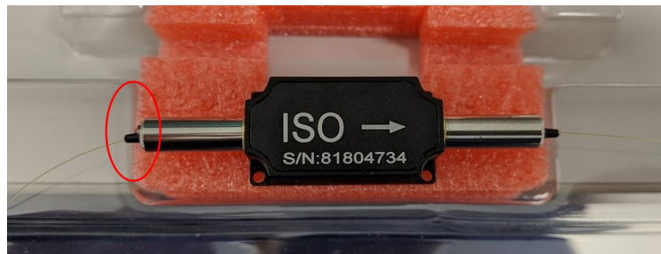
Figure 3.10: Photo of the pull-test failed isolator. It can be clearly seen that the strain relief boots have become loose (circled).
