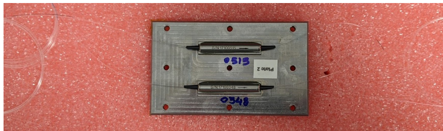
Figure 3.12: Photo of the returned non-PM hybrid components, post-fiber pull test.
