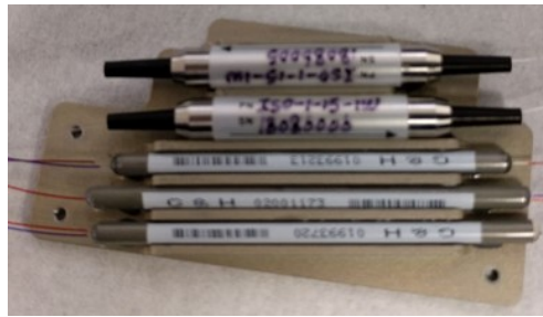
Figure 4.25: Fiber optic components fitted to CubeCAT fiber optic component carrier.
