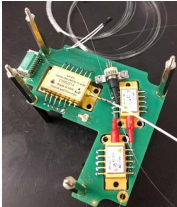
Figure 4.23: Photos of the fully assembled CubeCAT PCB ready for testing.
