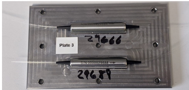
Figure 3.11: Photo of the returned PM hybrid components, post-fiber pull test.
