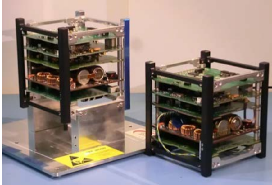
Figure 4.1: Photos showing the typical structure of 2 typical CubeSats (FUNcube). From: [4.7]
