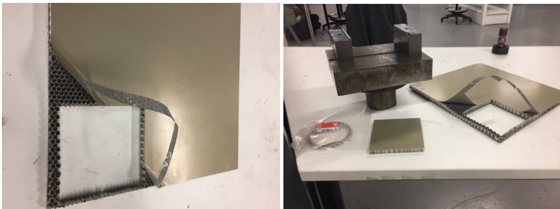
Figure 3.1. A honeycomb sandwich panel as typically used in the aerospace industry
