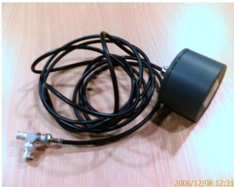
(a) Completed ILT (device B) in a watertight housing
