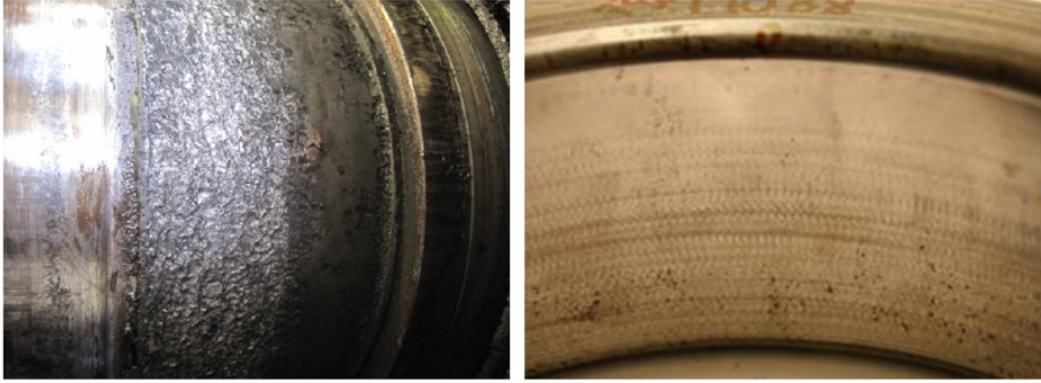
Figure 4.11: Damage to Generator bearing and shaft at time of replacement.
