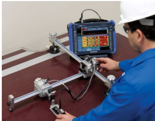
Figure 26- NDE Weld Pipe Scanner and X-Y Scanner [117, 118].
