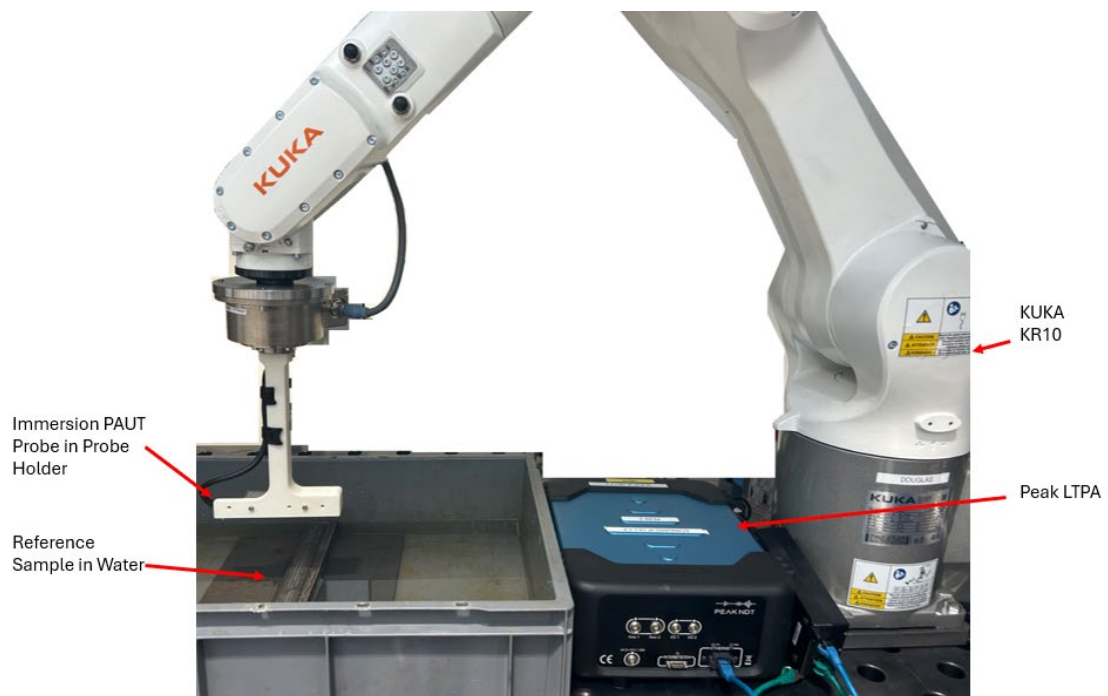
Figure 37 - Immersion Ultrasonic Equipment Set-Up
