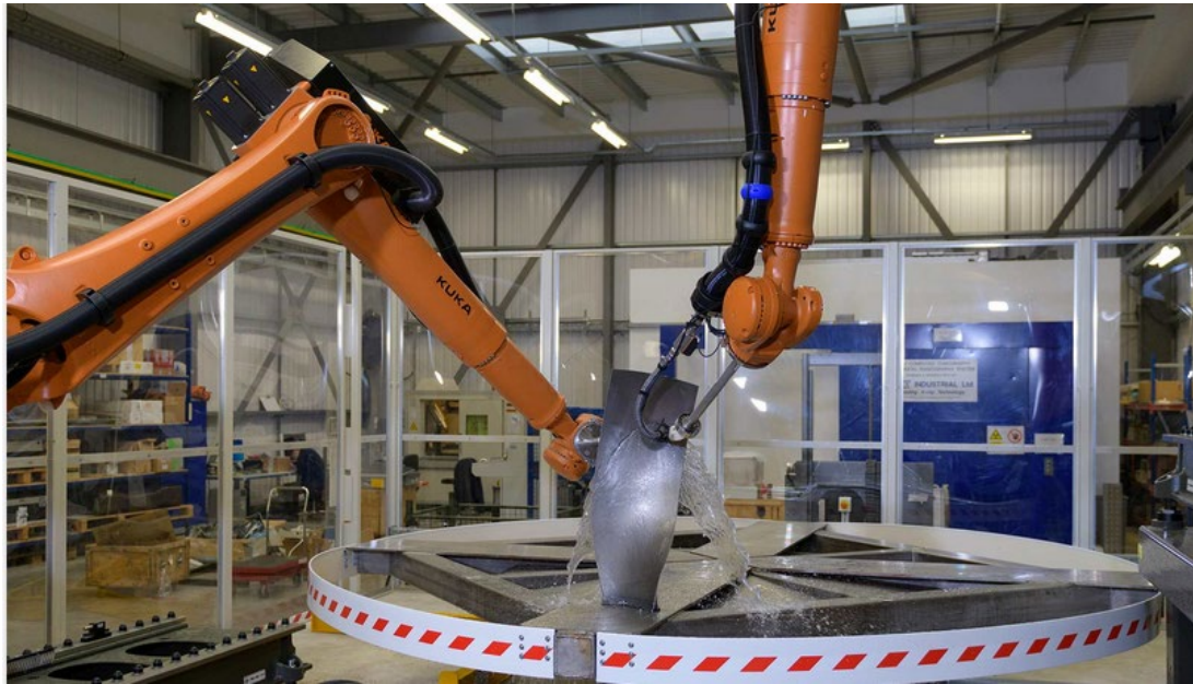
Figure 27- Robotic Arms Conducting Fan Blade Inspection [119].
