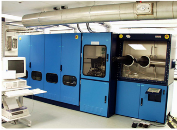
Figure 5.1: Image of the AIX 200/4 RF-S MOCVD system. Image courtesy: Ian W. Watson.
