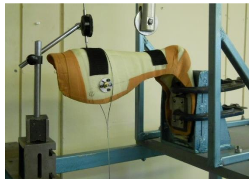
Figure 17: The surface area on which the measuring pen rested in compression testing.
