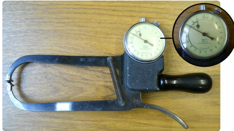
Figure 28: Thickness gauge used to measure the wall thickness of all four AFOs.
