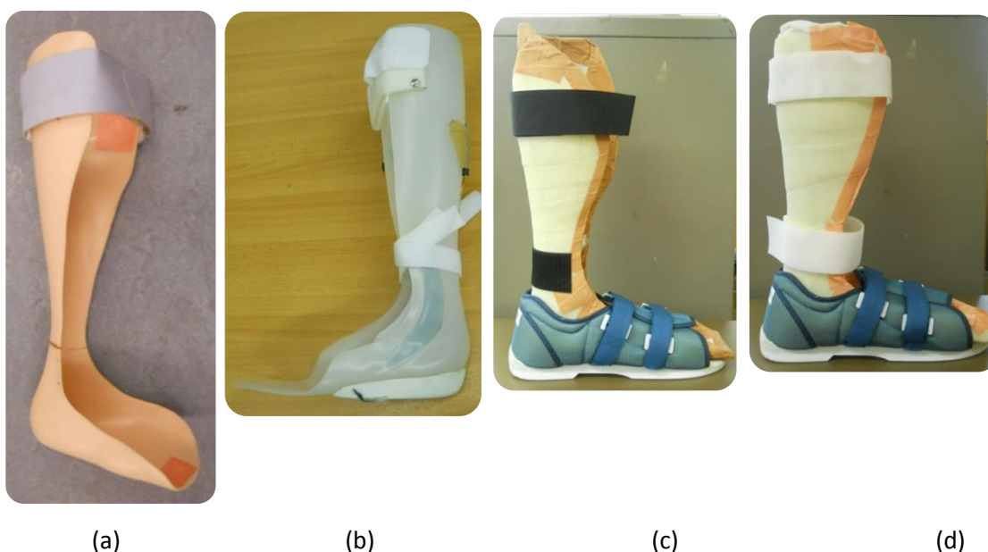
Figure 12: Set of orthopaedic AFOs, consisting of (a) 3.0 mm thick flesh coloured posterior leaf spring AFO, (b) white coloured solid AFO with carbon fibre reinforcement at the ankle section, (c) six layer SWIFT Cast, (d) eight layer SWIFT Cast, used in mechanical testing.
