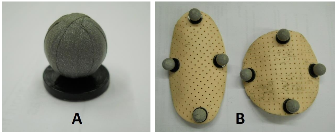
Figure 8: (a) Individual 14 millimetre retro-reflective marker, (b) Cluster marker for shank and thigh segments
