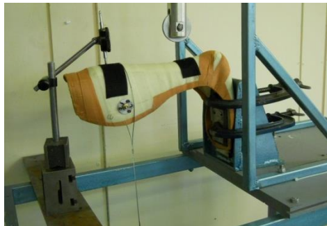
Figure 14: A representation of an orthosis mounted in a rigid metal frame with G-clamps for testing.
