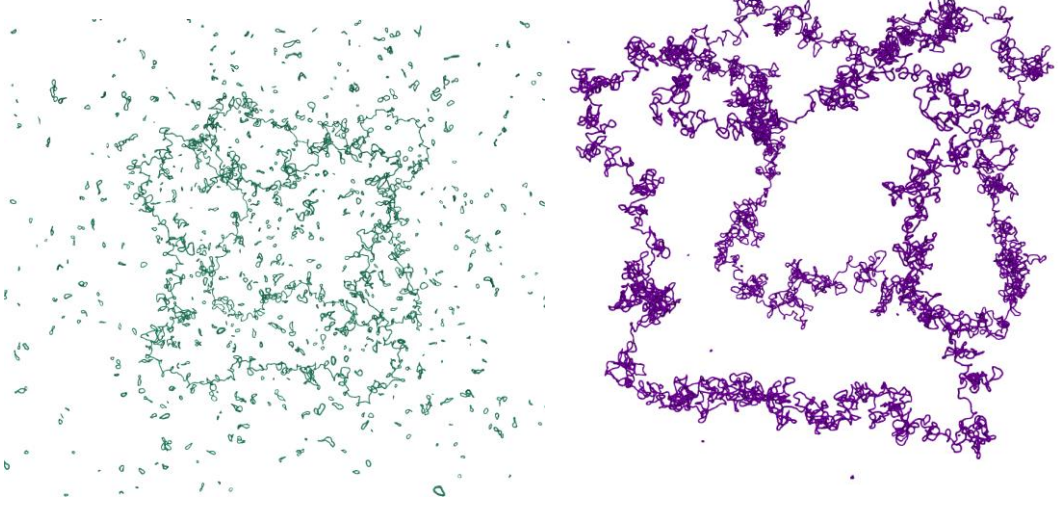
Fig. 27 - Cubic tangle configuration at t=20.11 when reconnections are allowed (left) and disallowed (right).
