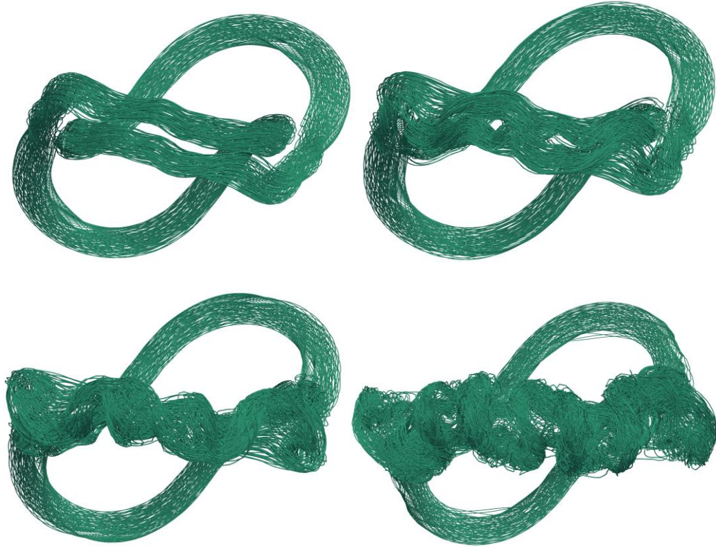
Fig. 68 - Crow instability generated and growing on the bridge portion of the Hopf-Link configuration at t=1.0647 (A), t=1.1408 (B), t=1.2168 (C) and t=1.3689 (D). At D, the instabilities have clumped up into a "secondary" bundle structure.
