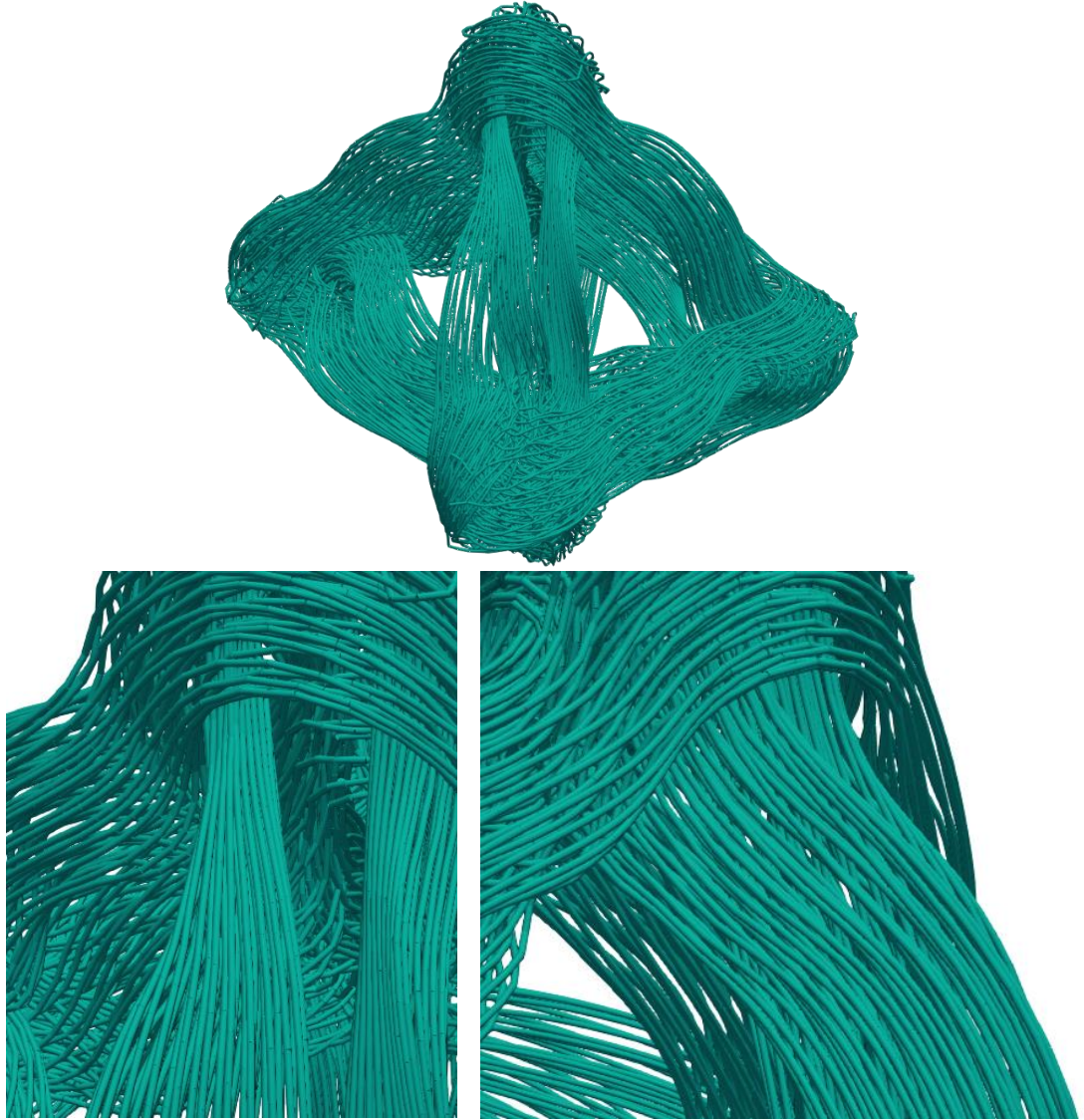
Fig. 48 – Quantized vortex tangle at t=0.1486 (top) and zoomed in section of a bundle front view (left) and side view (right).
