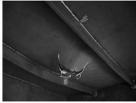
(c) Experimental study for the dropped object on a deck (Kozak, 2010)
