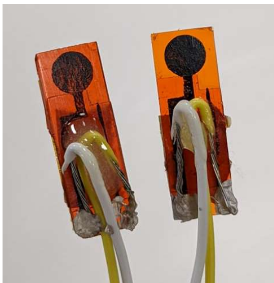
Figure 5.2: Discrepancies between MWCNT dispersion in two electrode chips. On the left-hand side, a lack of opacity can be observed, indicative of poor MWCNT network formation.
